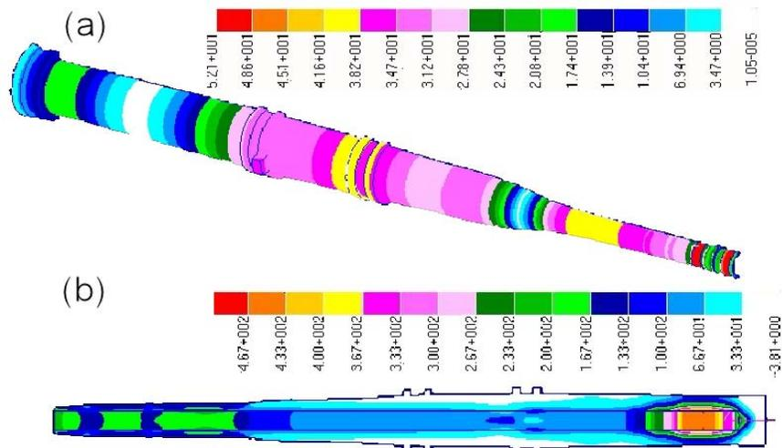
Figure 10 (a) shape change contours to tune transverse modes, (b) stress contours of improved shape
