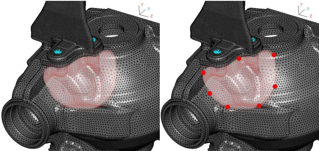
Figure 7 Active domain for reshaping the component, and the selected control points
