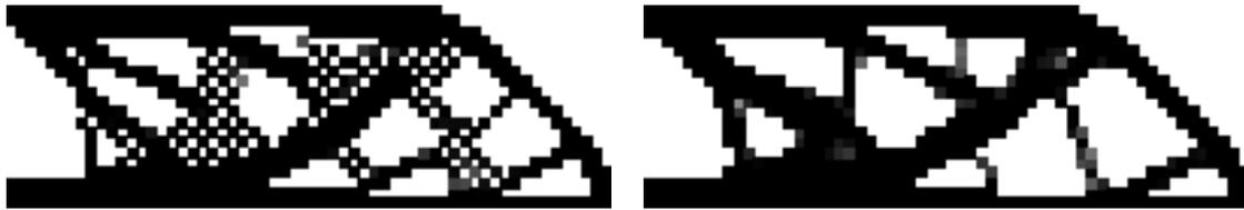
Figure 1 Checker boarding and checker board control models of a cantilever beam
