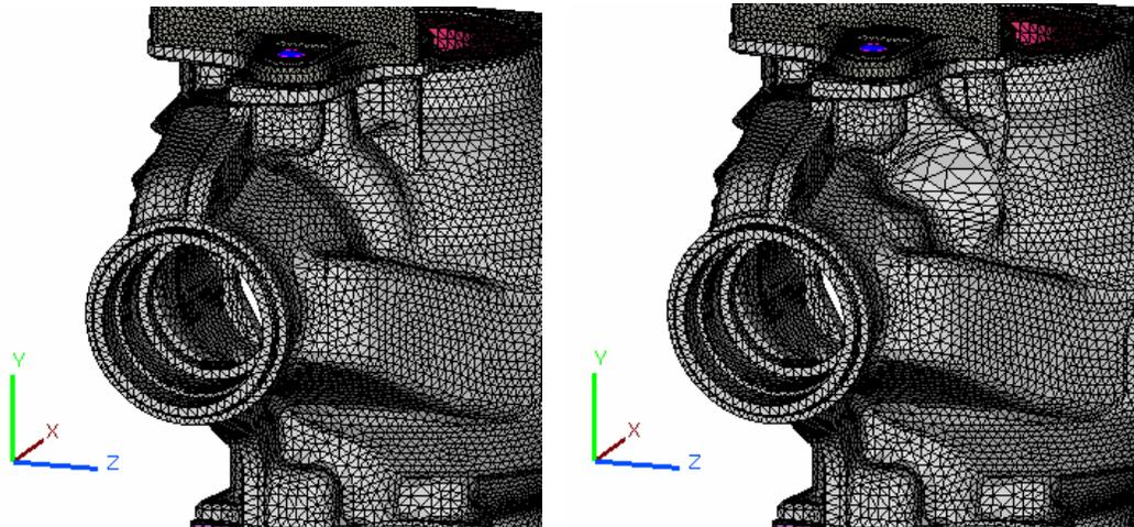
Figure 8 Before (left) and after (right) reshaping the first selected region
