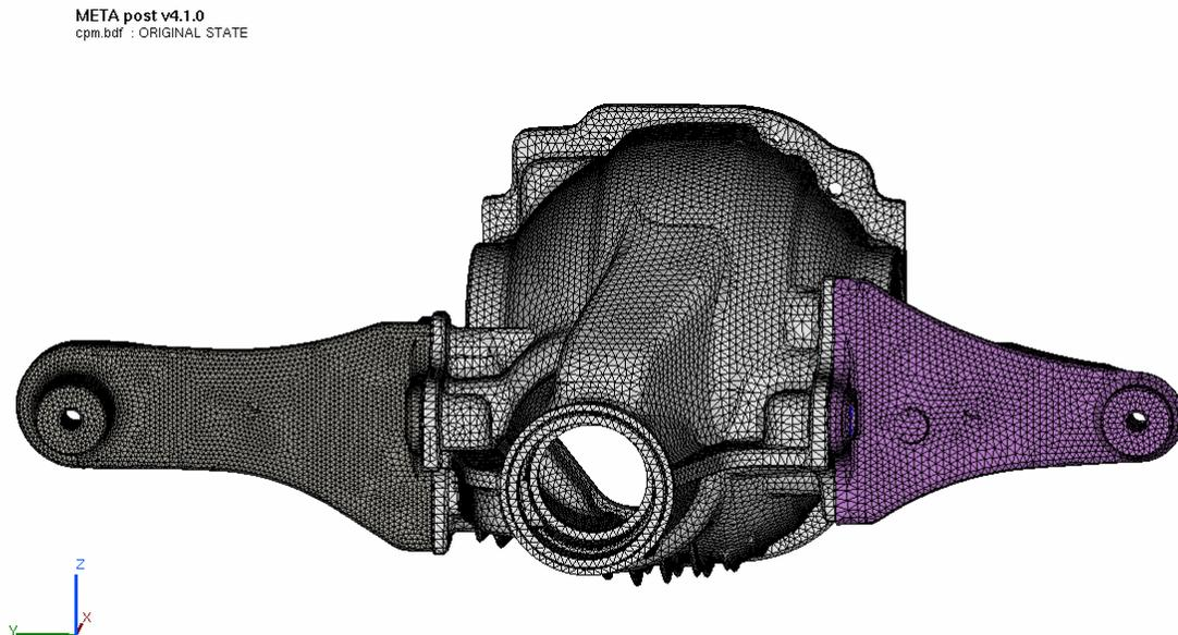
Figure 6 Differential case and bracket (Courtesy DANA Australia)
