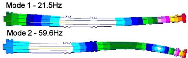
Figure 9 Displacement contours for transverse modes of vibration of the 16<sup>th</sup> century Spanish cannon
