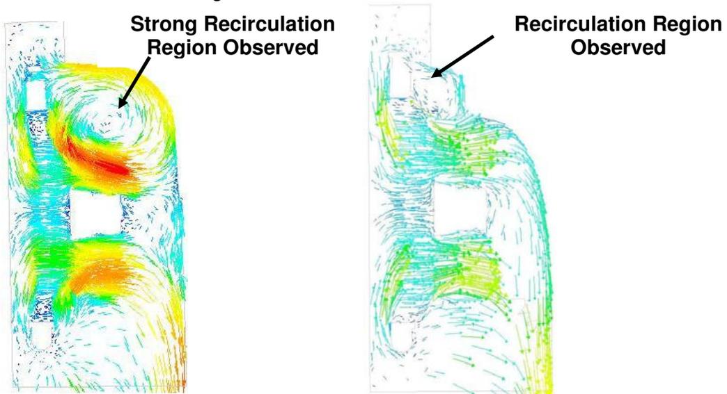
Figure - 2.7 Base Case Versus Case 2 - Air Flow across Radiator Cover Center Line
