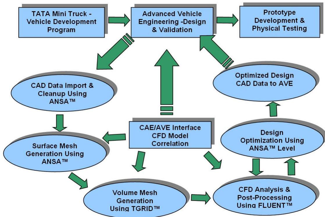
Figure - 2.1: Process for the Vehicle Development Program of TATA Mini Truck
