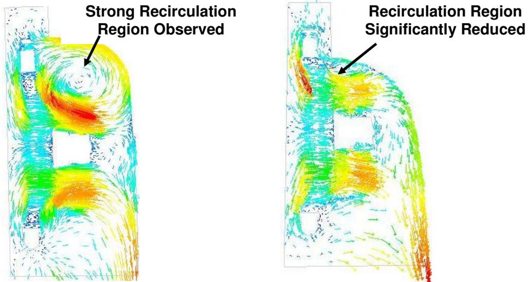
Figure - 2.8 Base Case Versus Case3 - Air Flow across Radiator Cover Center Line
