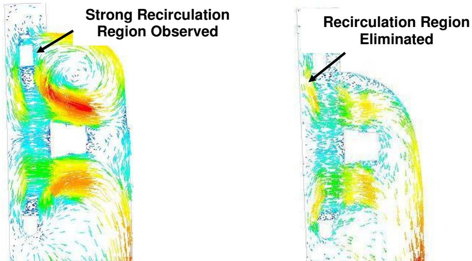
Figure - 2.9 Base Case Versus Case4 - Air Flow across Radiator Cover Center Line
