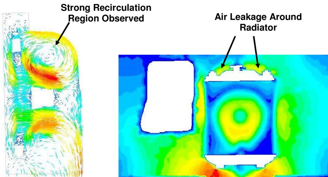
**Figure - 2.5 Base Case Air Flow Distributions across Radiator Cover Center Line**
