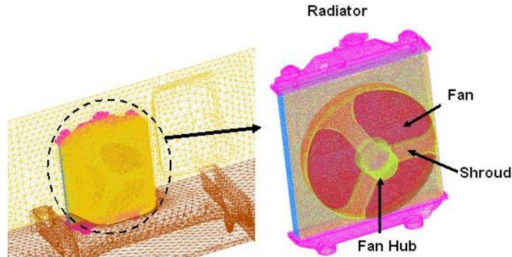
Figure – 2.3 Surface Mesh Generated By ANSA
