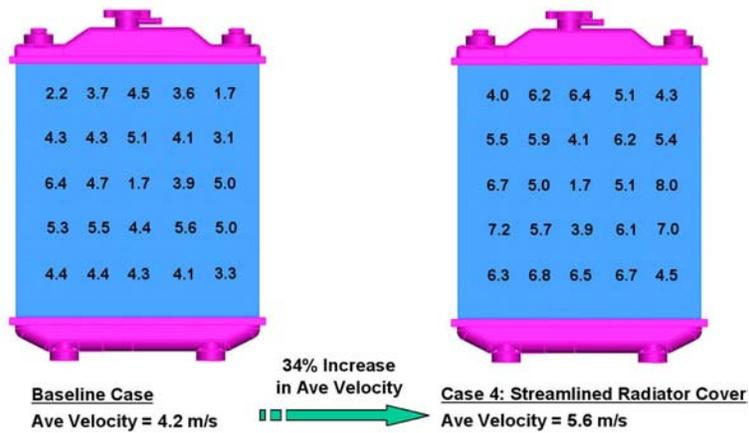
Figure - 2.11 Velocity Measured Locations on Radiator Face
