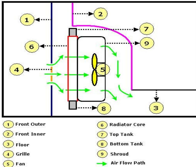
Figure - 2.2 Schematic of Radiator Assembly.
