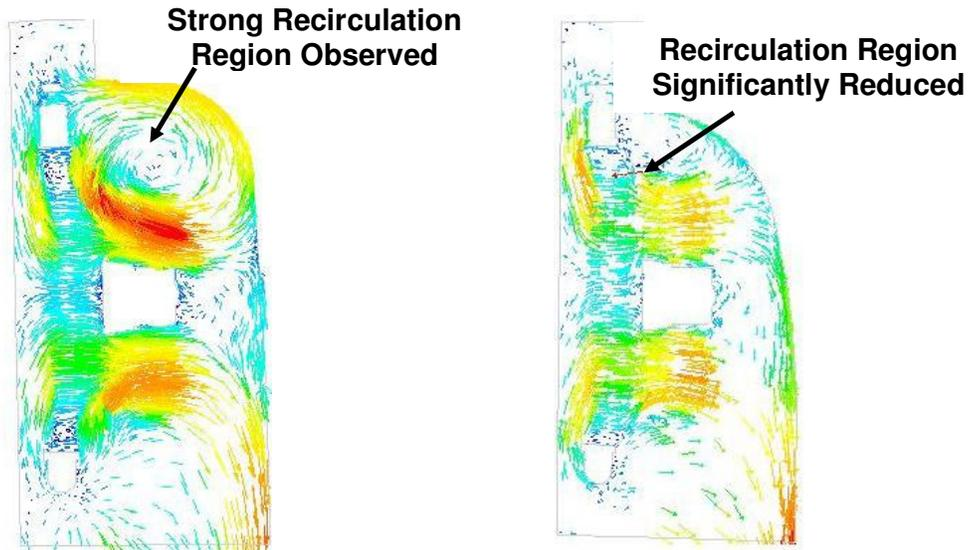
Figure - 2.6 Base Case Versus Case 1 - Air Flow across Radiator Cover Center Line
