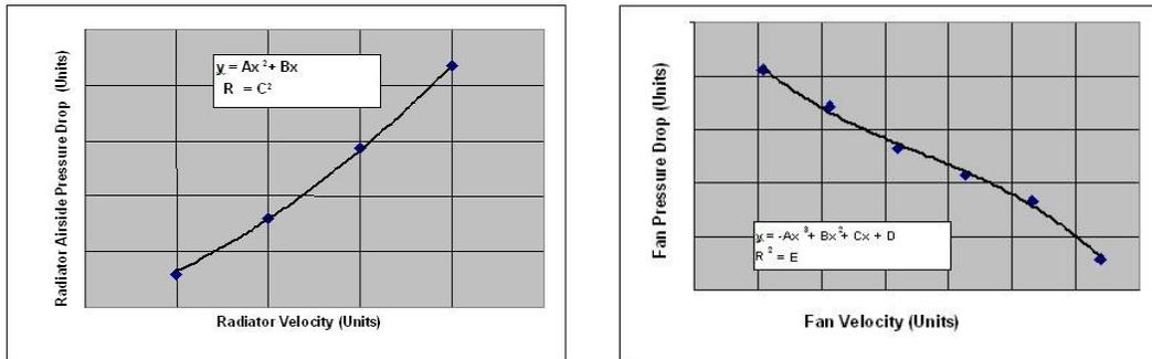
Figure – 2.4 Pressure Drop characteristics for Radiator & Fan
