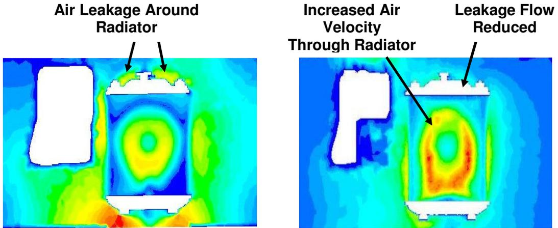
Figure - 2.10 Base Case Versus Case4 - Air Flow across Radiator face
