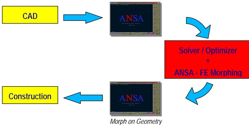
Fig. 18: Proposed solution combining both FE-model and geometry morphing.
