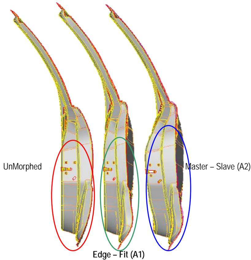
Fig. 12: Geometry Morphing, Case A1, A2 Rear View
