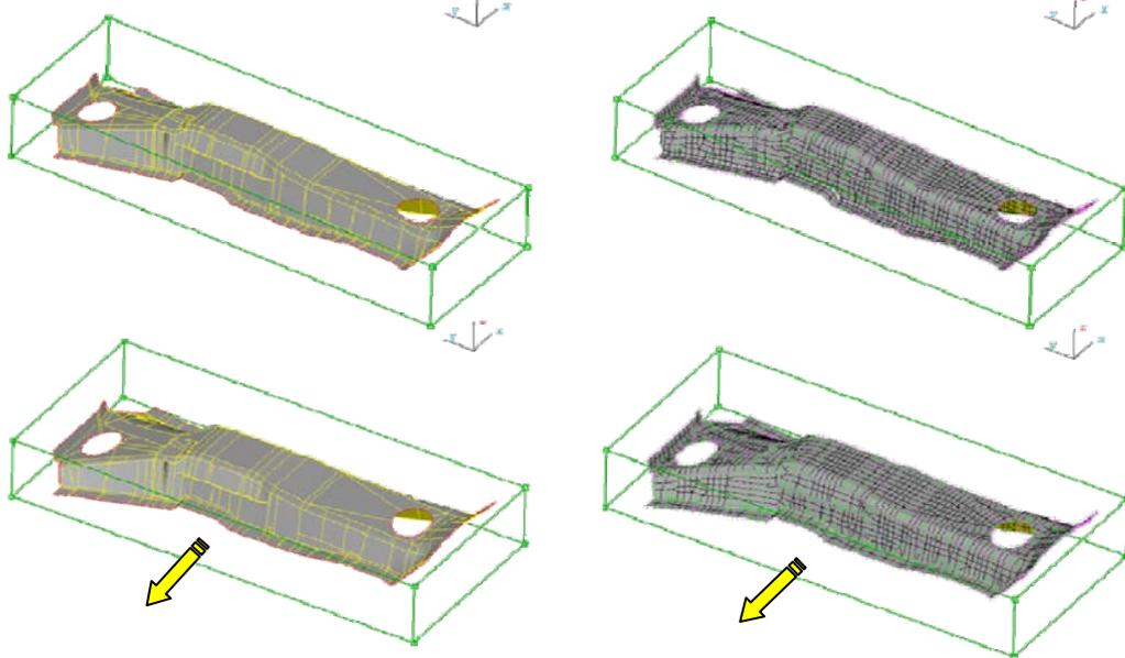
Fig. 6: During Geometry morphing the mesh on the faces is not lost, but it is morphed at the same time.
