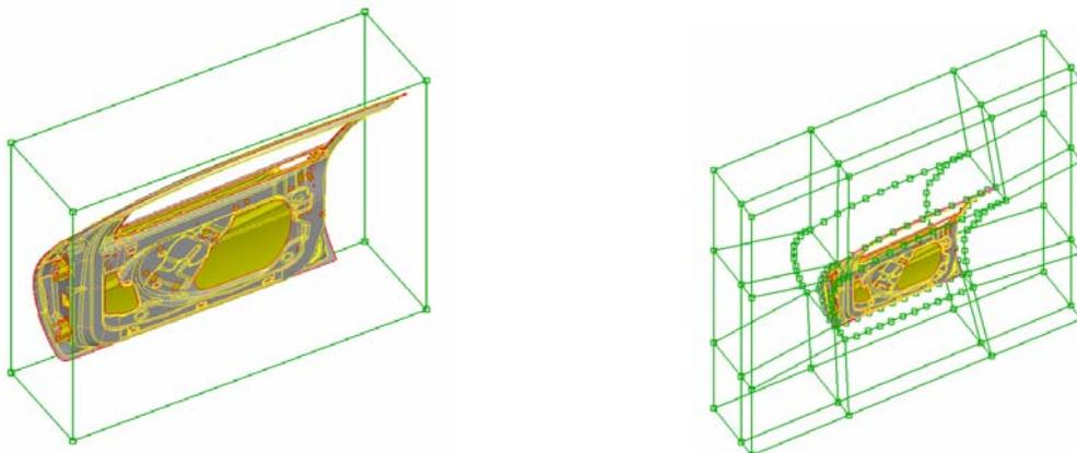
Fig. 9: Door assembly used for Geometry Morphing
