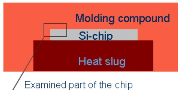
Figure 12: Longitudinal section of the examined object
