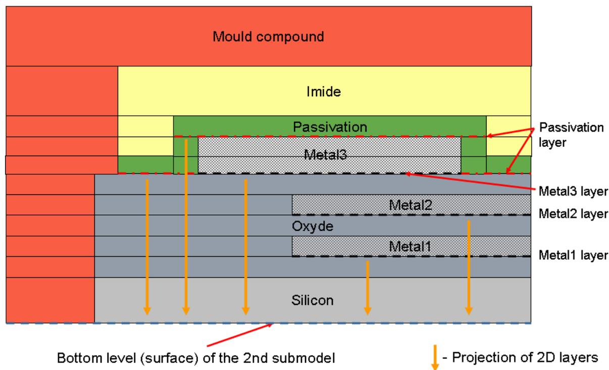
**Figure 24: Cross section through the 2<sup>nd</sup> submodel**
