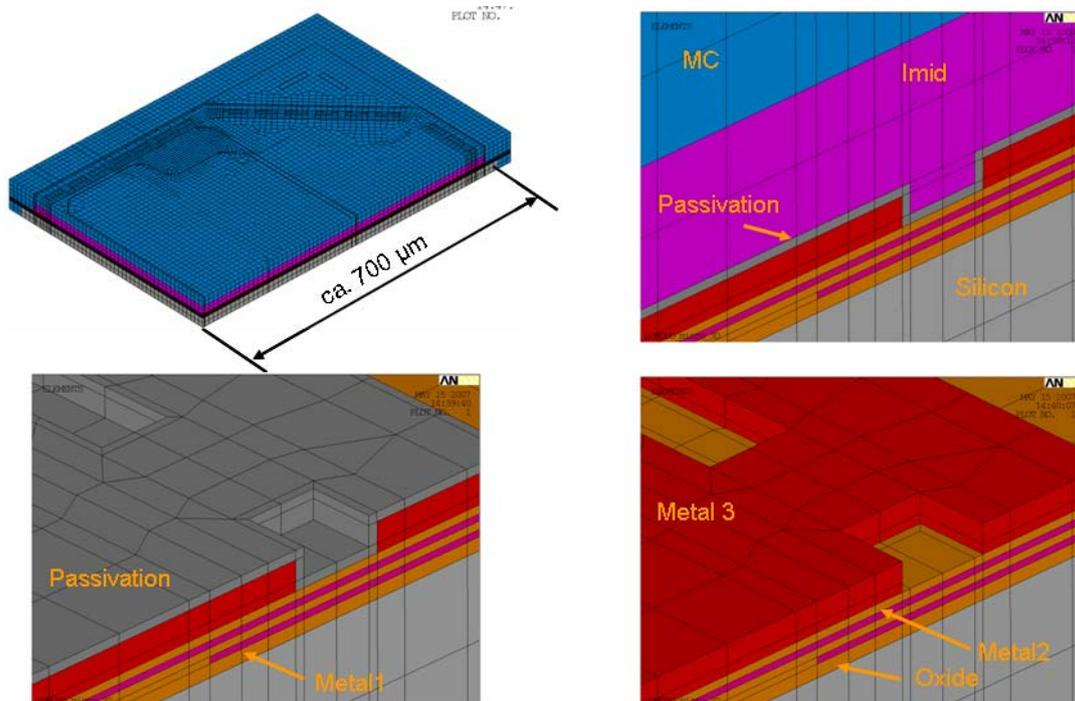
Figure 28: 3D FE-model of the crack region
