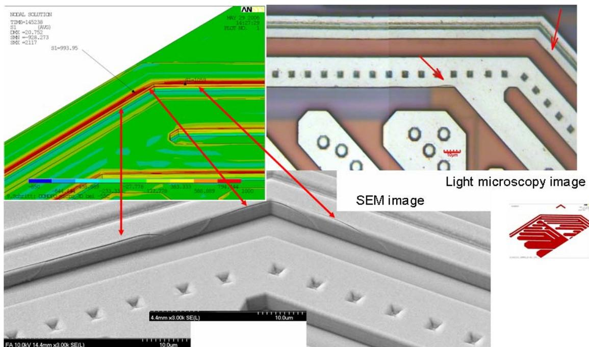
Figure 30: FE Results from 3D simulations compared with SEM Images
