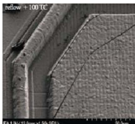
**Figure 16:** First visible cracks after 100 TC
