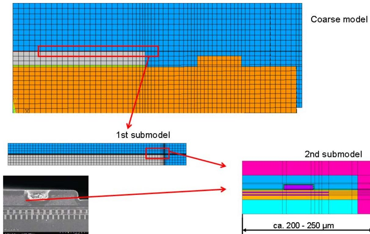
Figure 23: 2D-model of the chip – Coarse model, 1<sup>st</sup> and 2<sup>nd</sup> submodel
