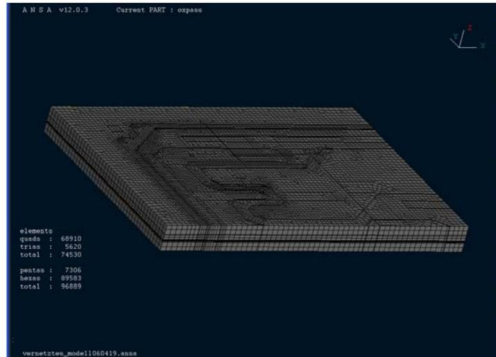
Figure 27: 3D FE-model generated by "step by step" extrusion
