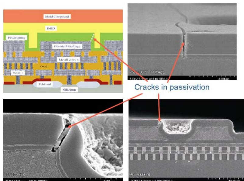
**Figure 14: Scanning electron microscopy images of passivation cracks**
