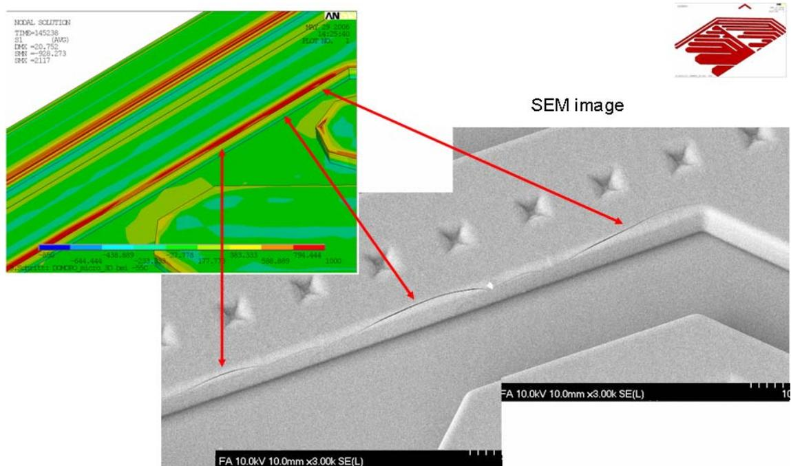
Figure 31: FE Results from 3D simulations compared with SEM Images
