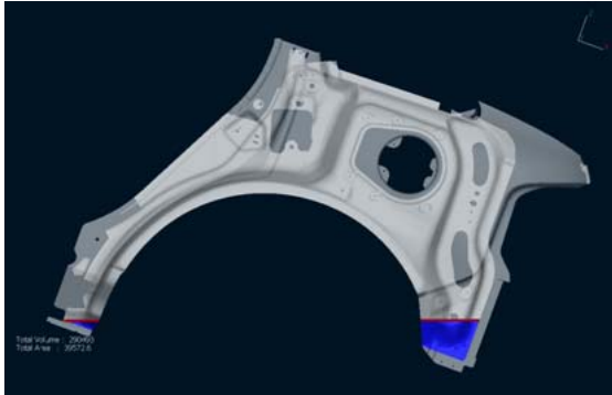
Figure 12: E-coat accumulation was identified by V.TRAPS.
