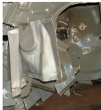
Figure 2: A prototype is cut open to measure e-coat film build inside the rocker.
