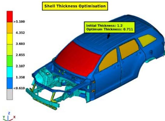
Figure 24 – Shell thickness results from design optimisation analysis
