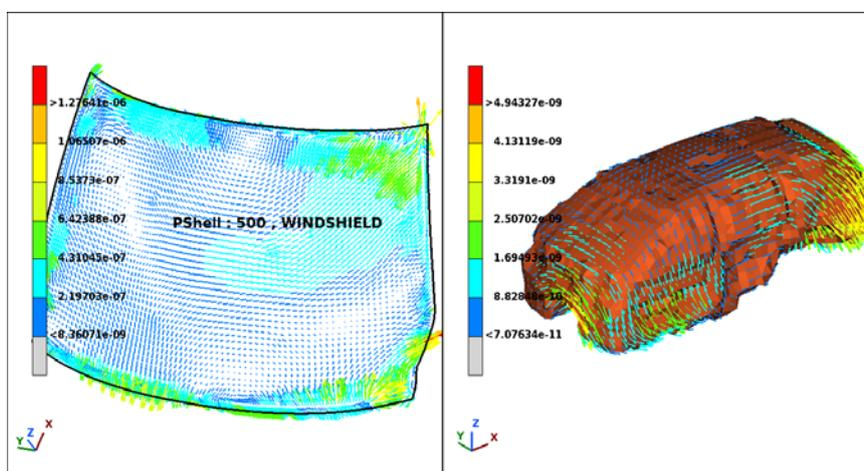
Figure 22 – Mechanical & Sound intensity results as a vector plot
