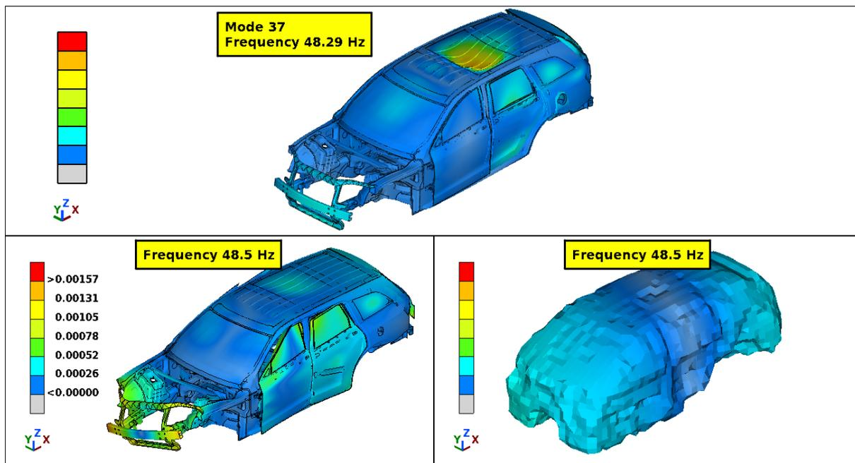
Figure 17 – Operating mode at 48.5 Hz and mode 37
