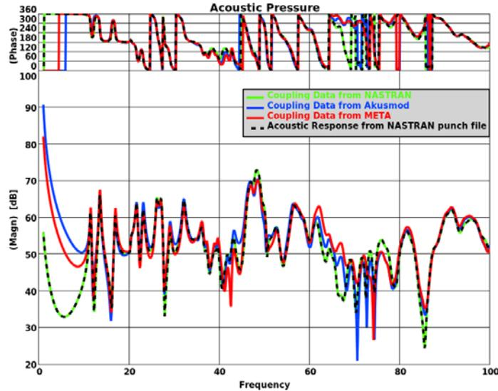
Figure 13 – Acoustic pressure for the same node and different coupling sets
