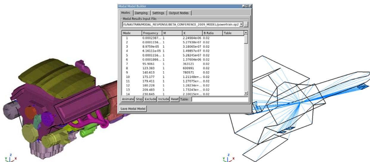
Figure 23 – Creation of the modal model for the power-train in META
