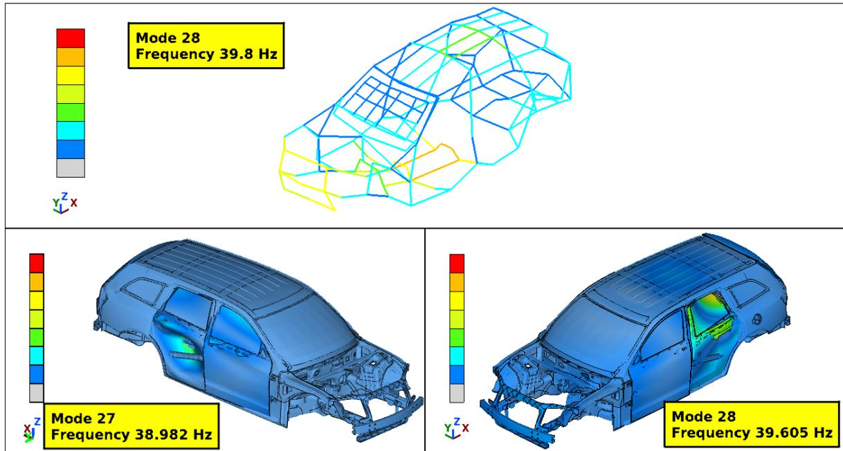
Figure 9 – Display / animation of multiple modes as different instances of the same model and the test model
