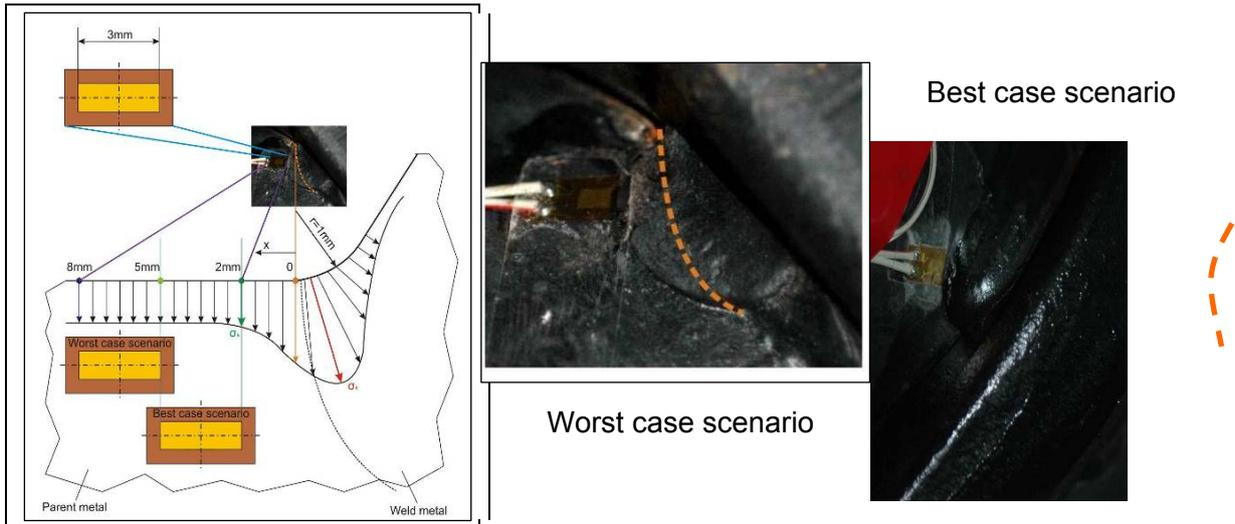
Figure 7 - Factor of distance of the applied strain gages - geometrical variation of weld-ends
