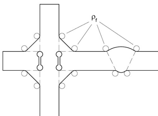
Figure 2 - Fictitious notch rounding (graph according to Hobbacher, 1996) [5]
