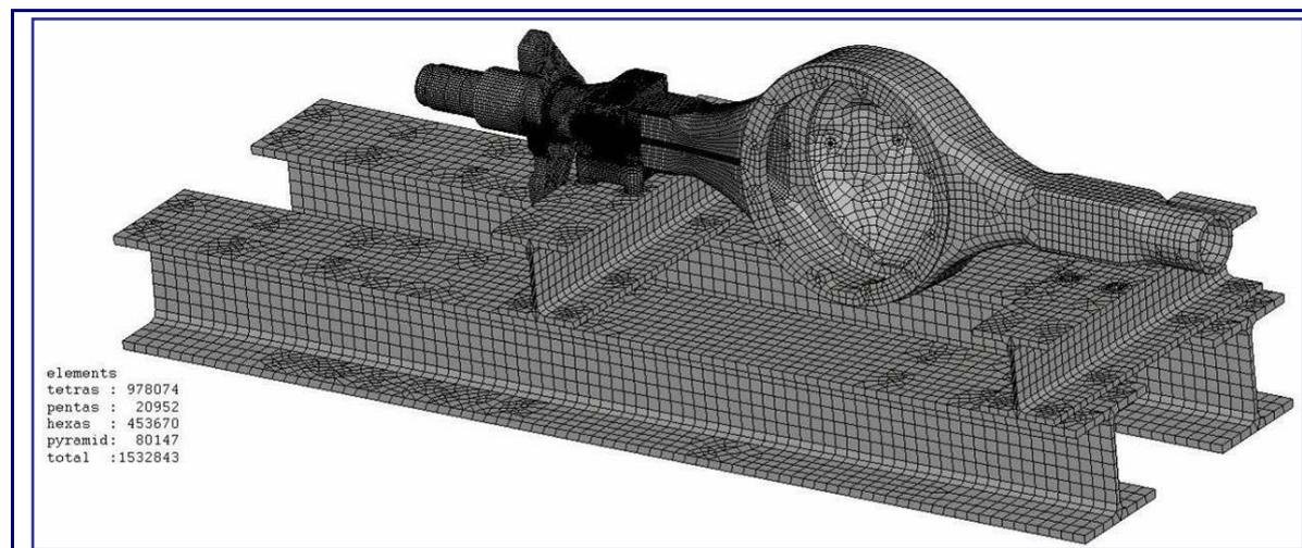
Figure 6 - Complete model – Test rig simulation
