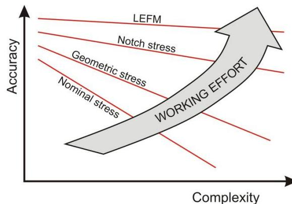
Figure 1 - Qualitative comparison of accuracy and effort for common fatigue assessment methods for welded structures (source: Marquis and Samuelsson [2, 3])
