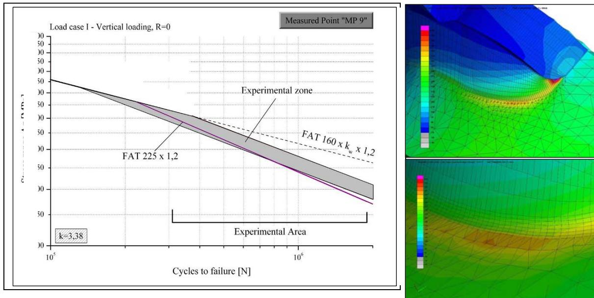
Figure 9 - Comparison between calculated and theoretical fatigue life curves with  $R=0$ , for the failure point of load case 1.
