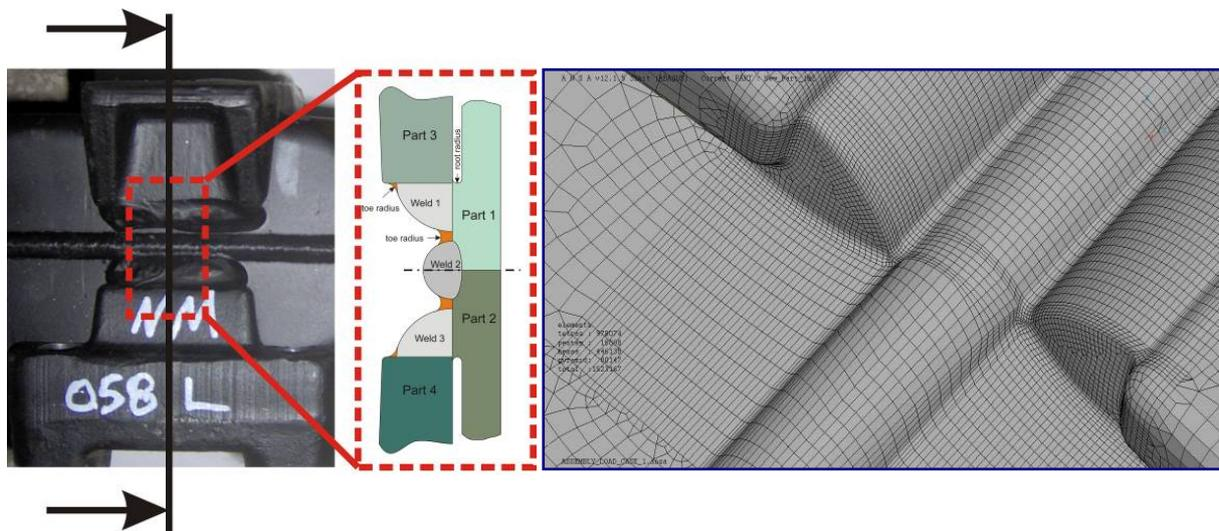
Figure 4 - Example of mesh created for the notch stress analysis with  $r_{ref} = 1\text{mm}$
