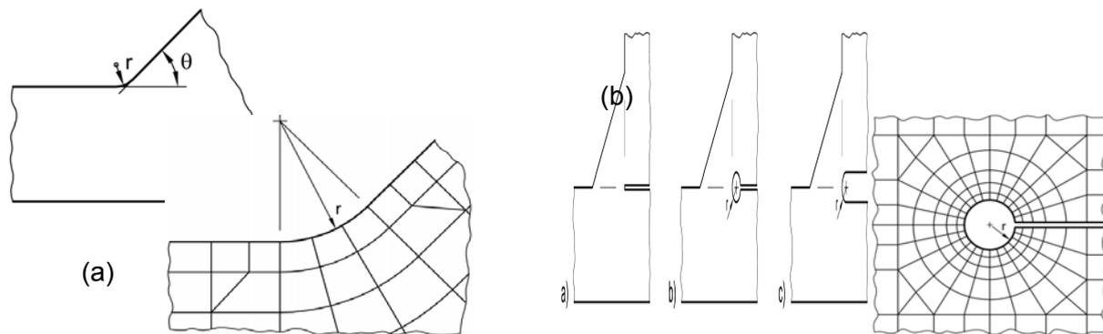
Figure 3 - Typical mesh for the notch stress analysis with elements having quadratic displacement function at the weld toe (a) and root (b) [5]
