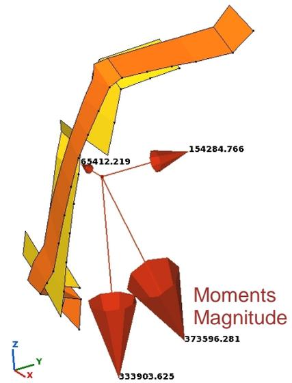
The vectors originate from the geometrical centre of the nodes assigned to the section. Subsequently, the Force and Moment results calculated by META are plotted against those of the LS-Dyna time history:
