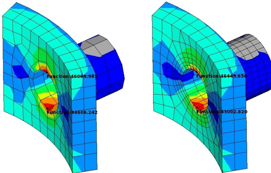
Solution comparison between coarse and fine meshed substructured area
