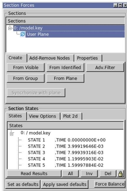
Sections can be created from *Visible* and *Identified* elements, from *Groups* (including Node Sets defined in the input deck), from existing *Planes* (including Sections defined in the input deck) and by specifying filtering criteria in the *Advanced Filter* tool of META.
