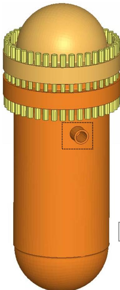
As an example, an ABAQUS-Standard finite element model of a reactor enclosure will be used.
