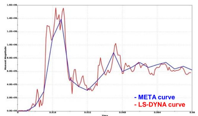
Some discrepancies between the two curves can be observed, however these are greatly reduced if the curves from the solver time history are filtered:
