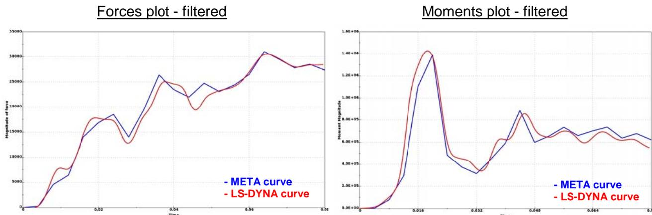
It is clear that the curves calculated by META closely follow those from the solver. Some peaks missed out are considered to be acceptable as the time interval for the calculation of the curve from META is much larger than that of the time history curve.
