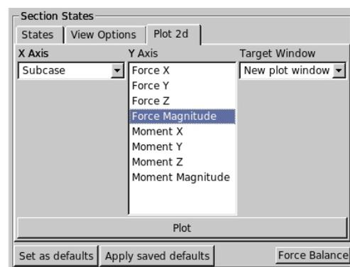
Using the above functionality the user is able to create a Section in any model region and accurately calculate Forces and Moments with accuracy comparable to those calculated by the solver within seconds. Thus, it is not necessary to define new Sections in the Pre-Processor and re-solve the Finite Element analysis, thus saving valuable time. Following is a verification of the accuracy of calculations performed in this field by META, against results extracted by the supported solvers.
