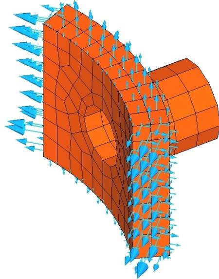
Freebody Loads assigned to the area to be substructured
