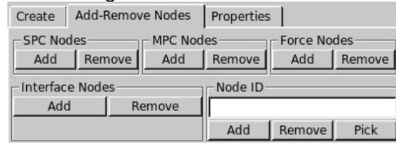
SPC, MPC, Force, Interface and user-specified nodes can be assigned to a Section in one step.
