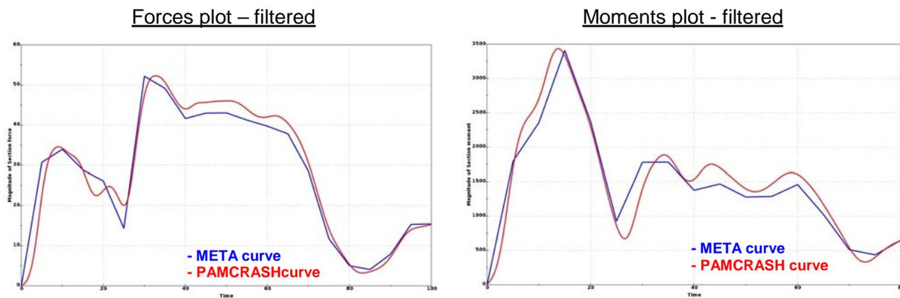
Having verified that the accuracy of the Forces and Moments calculated by META closely match those calculated by the solver, for existing sections, it is safe to conclude that this will be the case for Sections defined in META. This prevents the re-solving of crash models for sections not defined, making META a valuable Post-Solution calculator.
