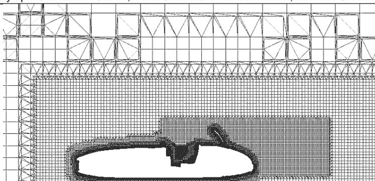
Figure 4 – Resulting volume mesh
