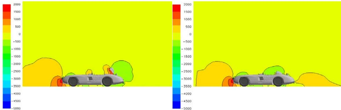
Figure 6 – Static pressure contours of the vehicle in close proximity to ground with (left) and without (right) the airbrake in operation.
