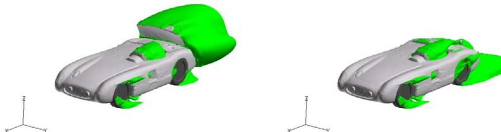
Figure 7 – Total pressure = 0 isosurfaces of the vehicle in close proximity to ground with (left) and without (right) the airbrake in operation
