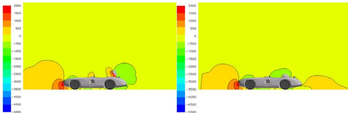
Figure 6 – Static pressure contours of the vehicle in close proximity to ground with (left) and without (right) the airbrake in operation.
