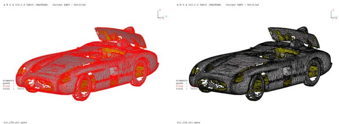
Figure 2 – Resulting geometry after scan, left highlighting unconnected STL geometry, right showing the how severely bad the scanned result was.
