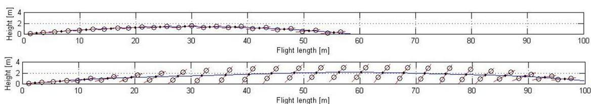
Figure 9 – Example showing a calculation with and without aerodynamic effects, the upper figure shows without the action of aerodynamics on the airborne vehicle, the lower shows with the action of aerodynamics.
