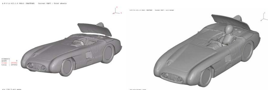
Figure 3 – Repaired and cleaned geometry to the left. To the right with a driver model added.
