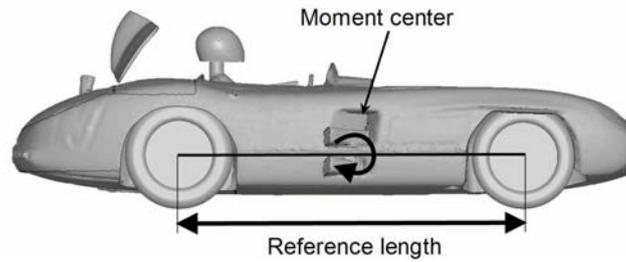
Figure 5 – Pitch axis definition
