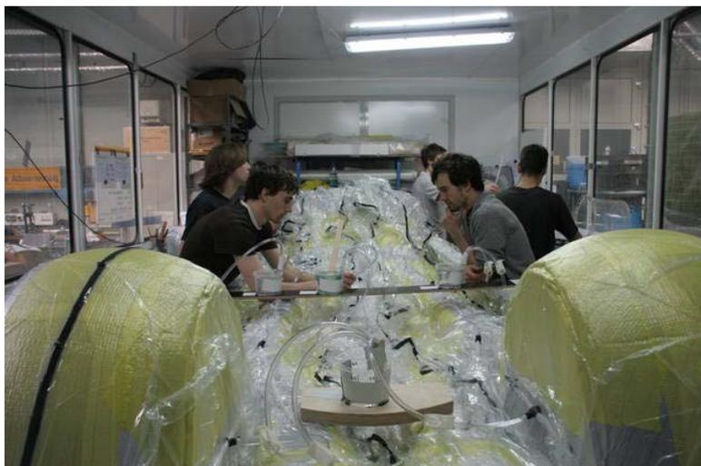
Figure 11 – Production of the ground body with vacuum infusion process
