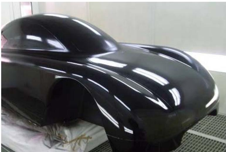
Figure 10 – Painted styrofoam body
