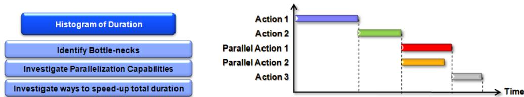
Figure 9 – Process profiling
