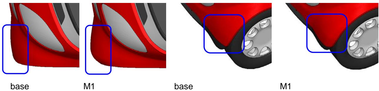
Figure 17: Morphing of the front fender to alter its curvature, top view (left) and isometric view (right)
