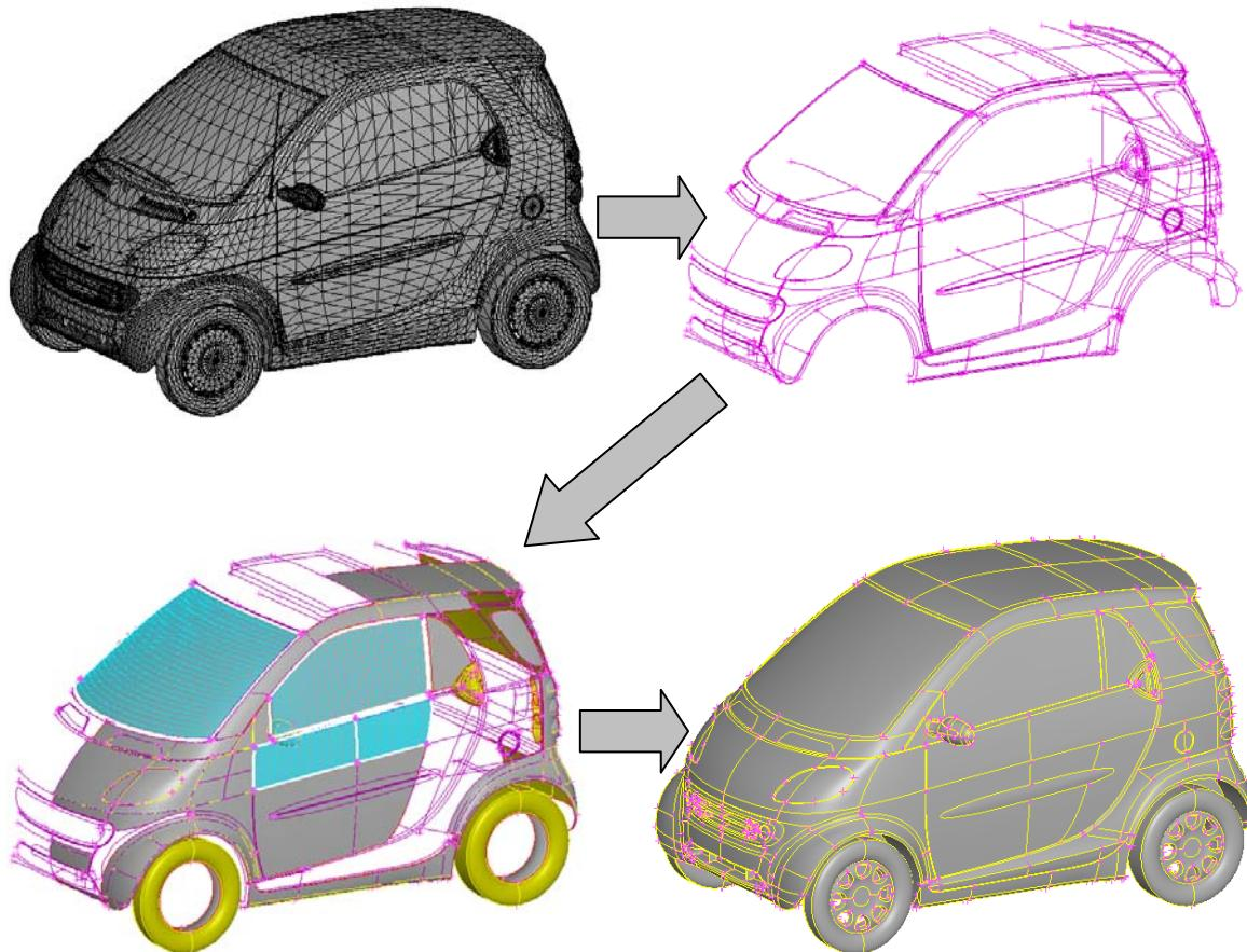
Figure 1: Geometry creation based on the STL input
