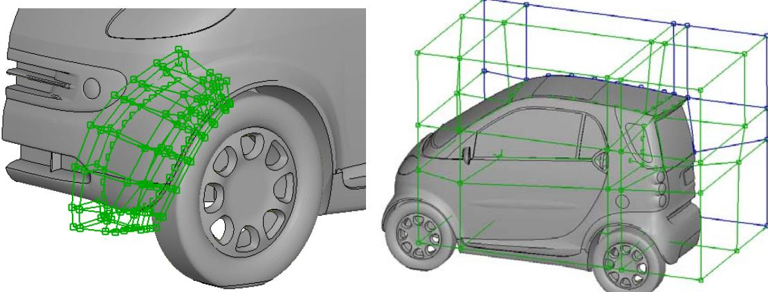
Figure 16: Morphing Box templates for the modification of the front fender (left) and the rear roof (right)
