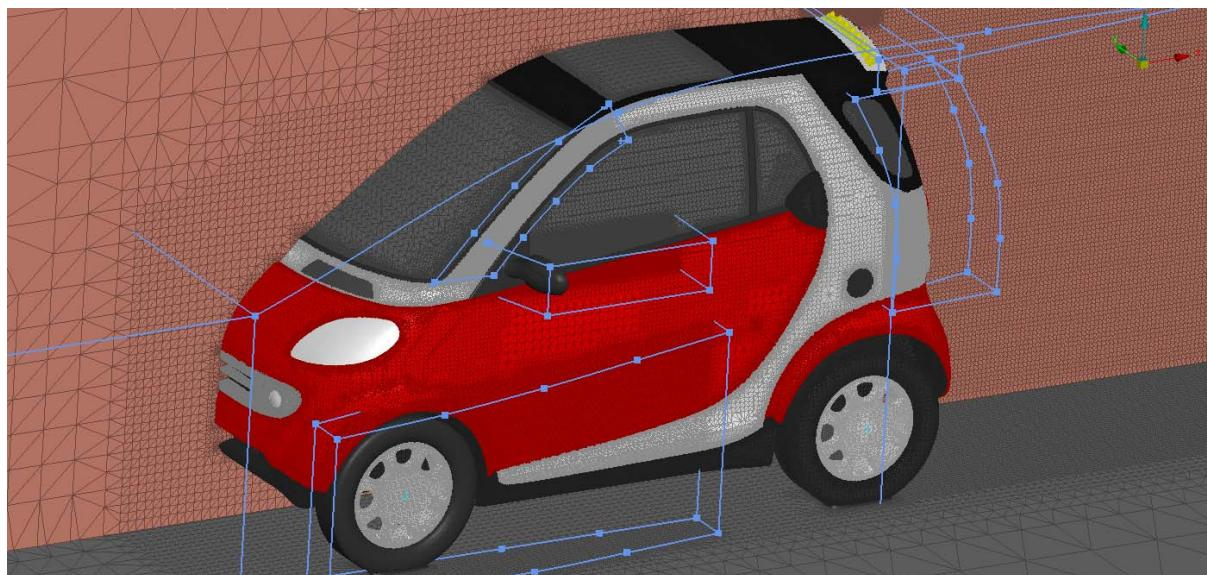
Figure 10: Surface Wrapping mesh
