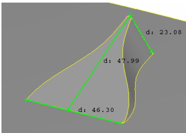
Figure 4: Close up and dimensions (in mm) of a VG
