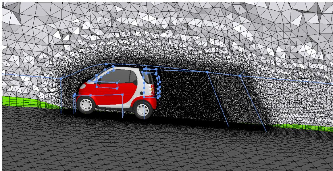
Figure 14: Section of the tetra mesh with the Size Boxes – 22 million elements
