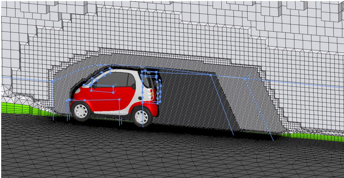
Figure 15: Section of the Hexa-Interior mesh with the Size Boxes – 9 million elements
