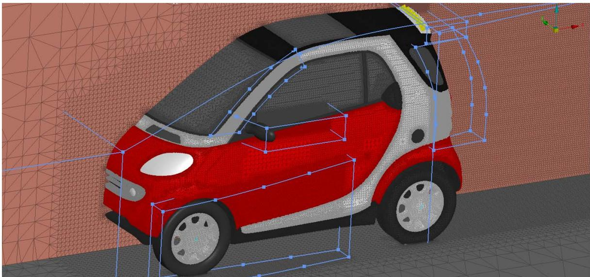
Figure 10: Surface Wrapping mesh
