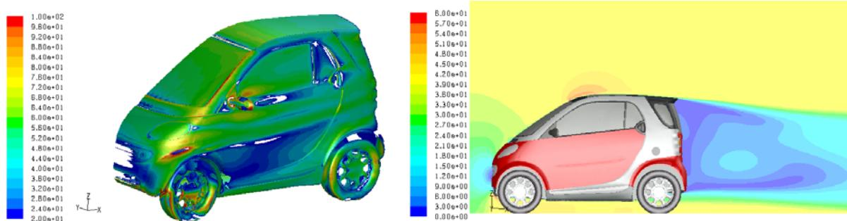
Figure 21: Contours of  $y^+$  in the range of 20 to 100 (left) and velocity magnitude contours on the symmetry plane (right) for base model
