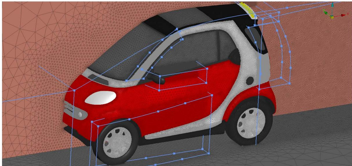
Figure 11: Surface wrapping mesh after quality improvement step
