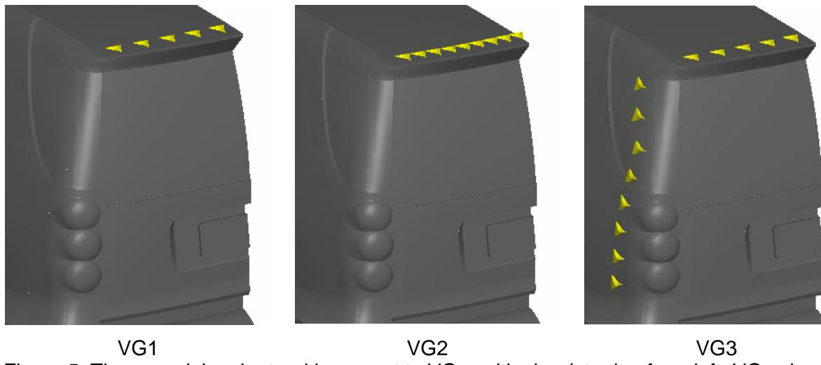
Figure 5: Three model variants with respect to VG positioning (starting from left, VGs placed on top, on top dense, and on top and sides)
