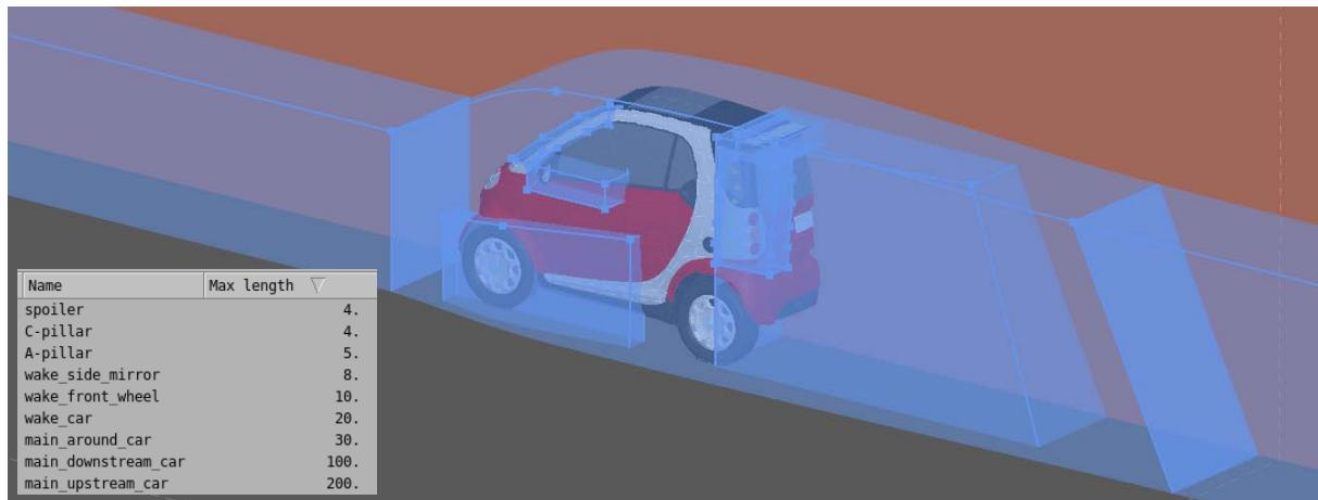
Figure 7: Size Boxes and corresponding maximum element length values
