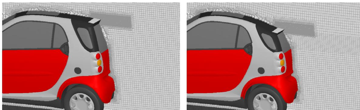
Figure 19: Morphing of the volume mesh model for M3 variant
