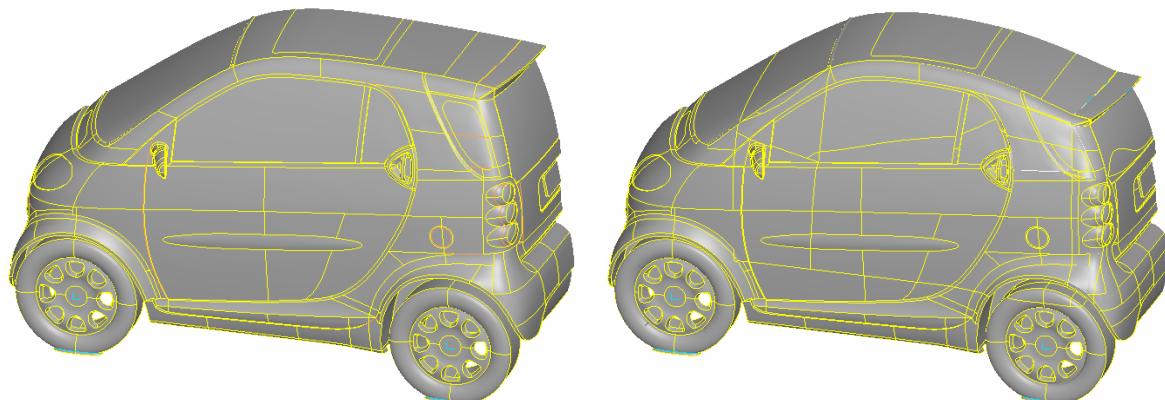
Figure 20: Original and morphed geometrical data for M3 variant
