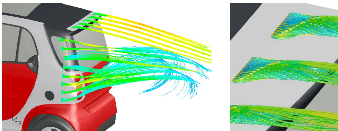
Figure 22: Streamlines coloured by velocity magnitude, released from the VGs for model VG3 and close up of the vortex formation around them
