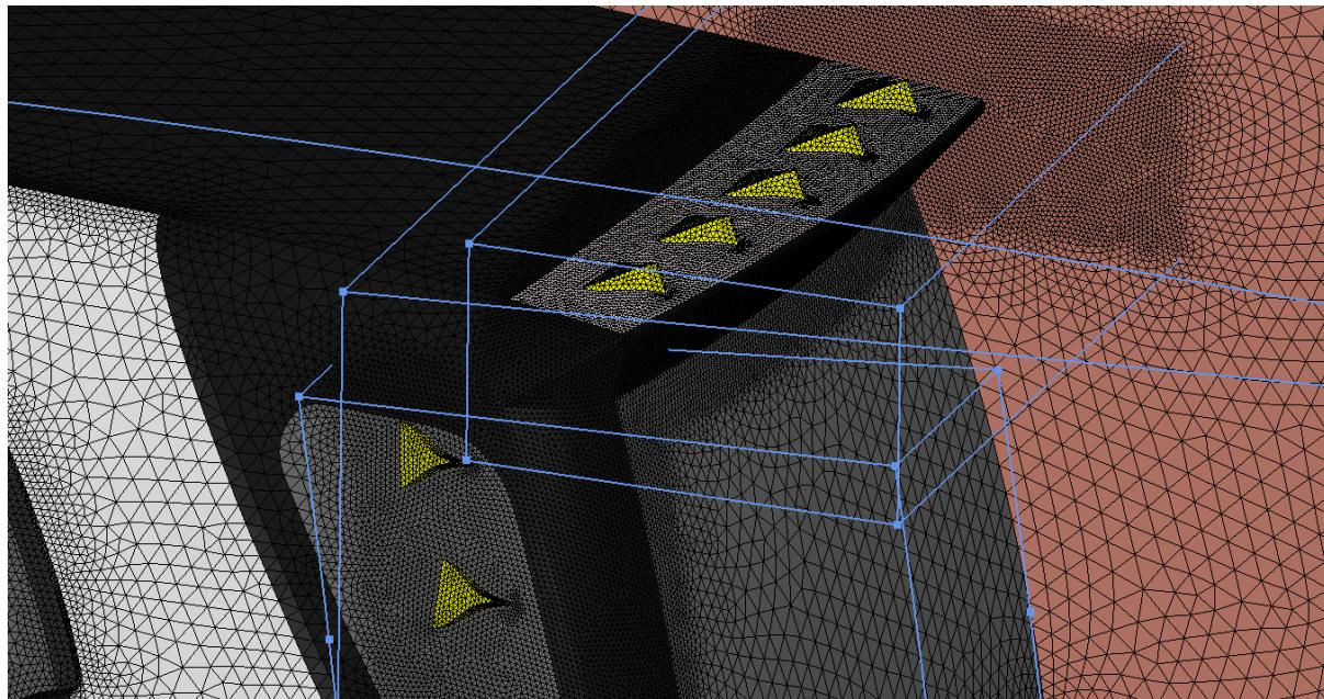
Figure 9: Close up of the surface mesh at the rear spoiler area showing the VGs
