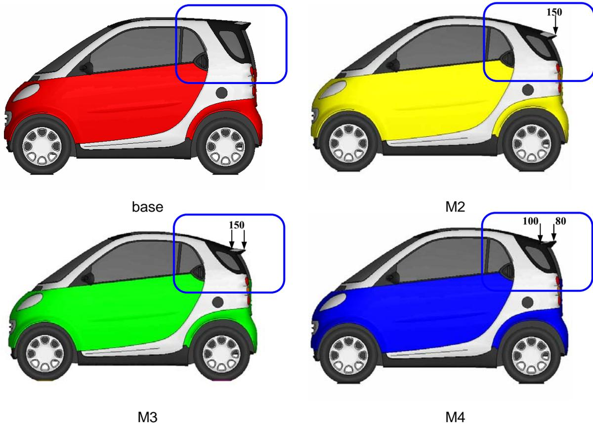
Figure 18: Imposed deformations, in mm, on the rear roof end for the three variants (Red is base model)
