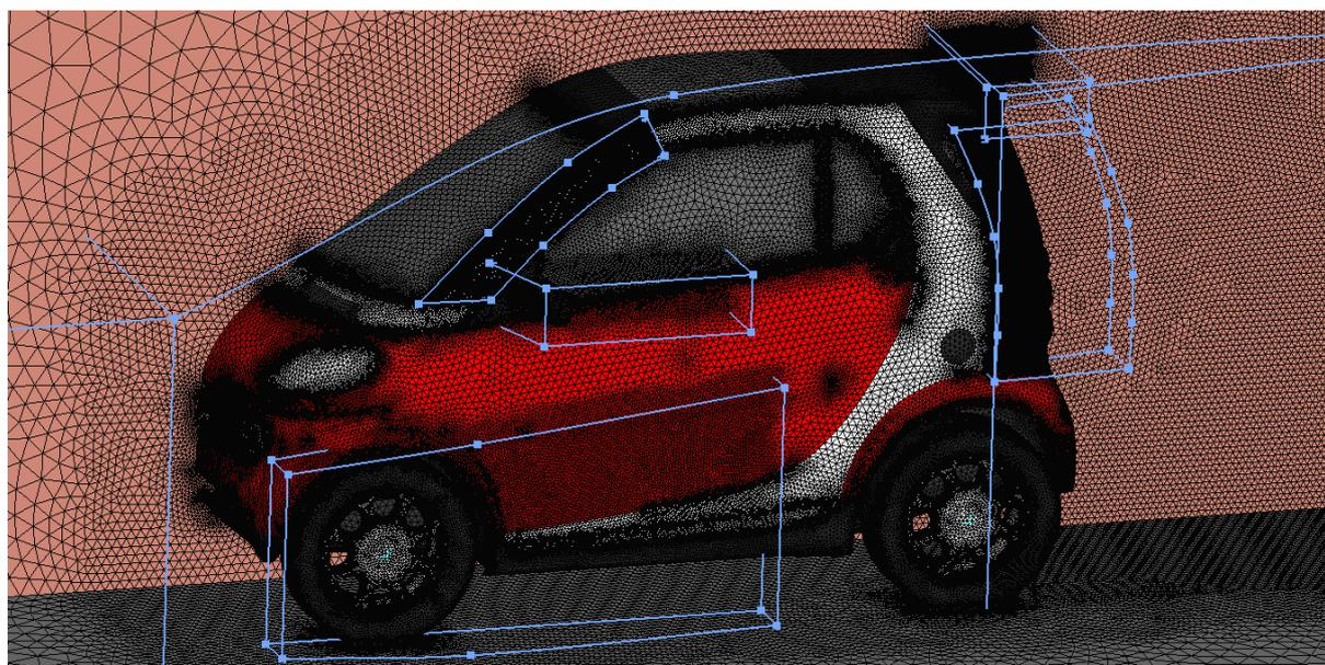
Figure 8: Surface mesh of approximately 452 thousand triangles, as created by batch mesh tool
