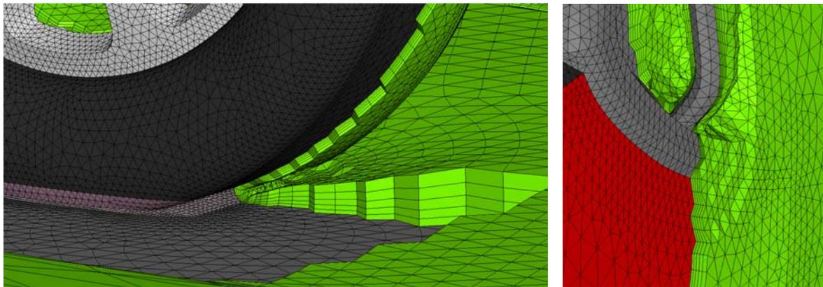
Figure 12: Close up of the layers near the tyre and road and around the door handle
