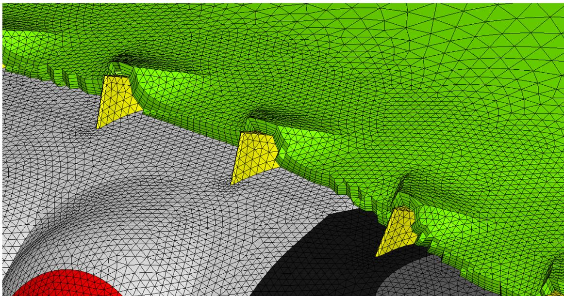
Figure 13: Close up of the layers around the side VGs
