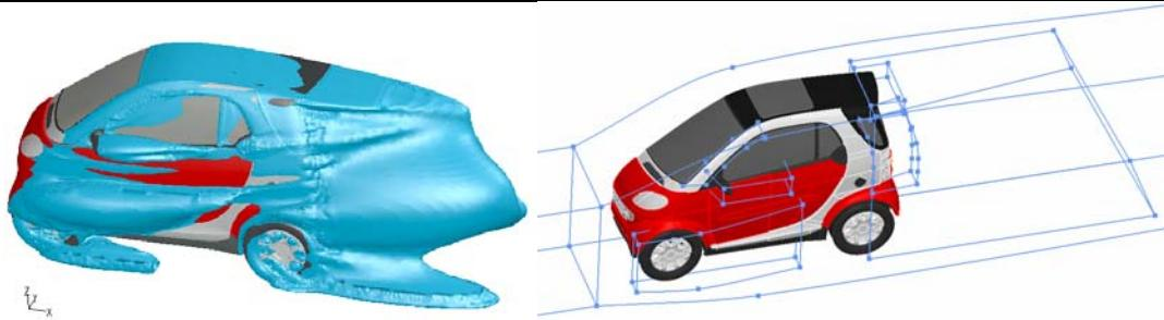
Figure 6: Iso-surface of total pressure equal to zero, as calculated in base CFD run (left) and final constructed Size Boxes for local mesh size control
