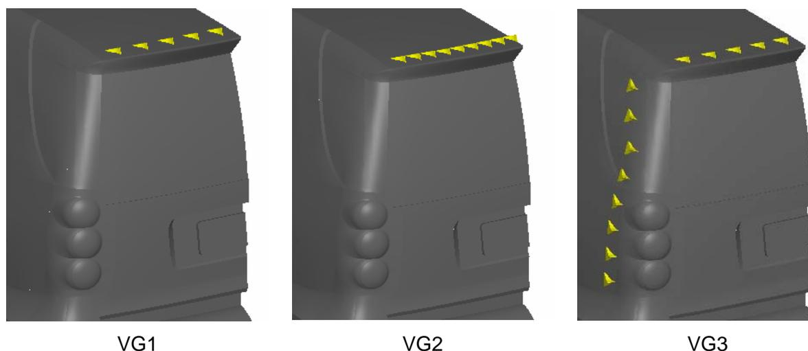
Figure 5: Three model variants with respect to VG positioning (starting from left, VGs placed on top, on top dense, and on top and sides)
