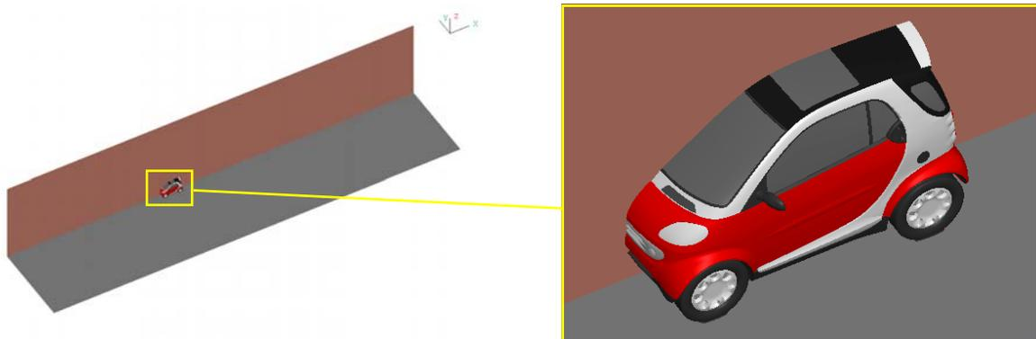
Figure 3: Computational domain and close up of car model
