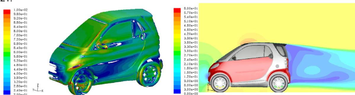
Figure 21: Contours of  $y^+$  in the range of 20 to 100 (left) and velocity magnitude contours on the symmetry plane (right) for base model
