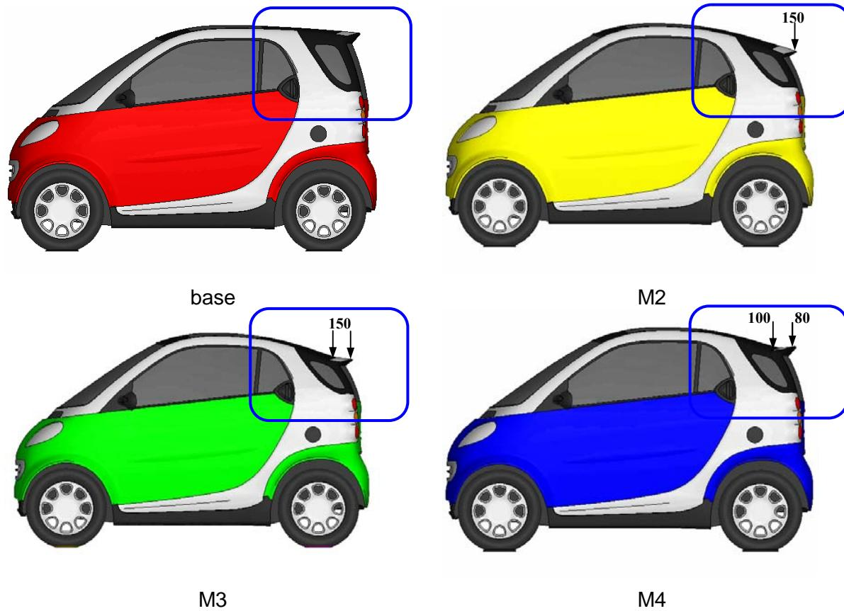
Figure 18: Imposed deformations, in mm, on the rear roof end for the three variants (Red is base model)
