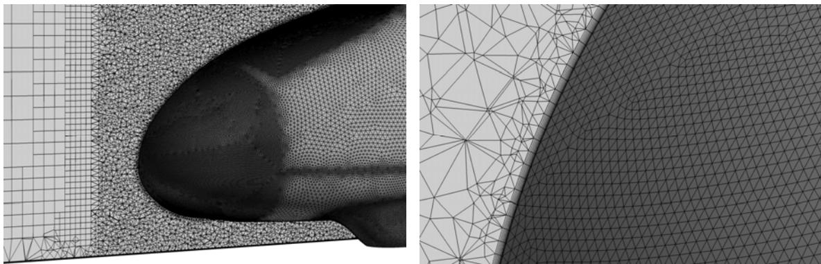
Figure 11 – A cut-out of the mesh. On the right a zoom-in image displays the 10 layers of prism cells.
