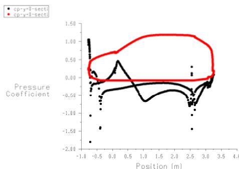
Figure 5 – Centreline pressure coefficient for the VRAK.
