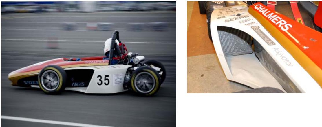
Figure 6 – The 2007 Chalmers formula student car and on the right a close-up on the right sidepod where the radiator is located.
