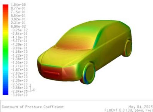
Figure 2 – Surface pressure coefficients on the VRAK.
