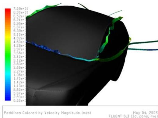
Figure 3 – Streamlines attempting to capture a-pillar vortex structure.
