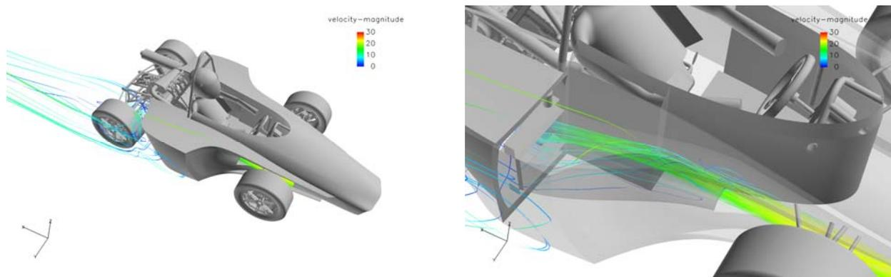
Figure 9 – Streamlines illustrating the improved cooling flow.
