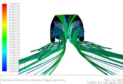
Figure 4 – Streamlines in the wake of the VRAK model.
