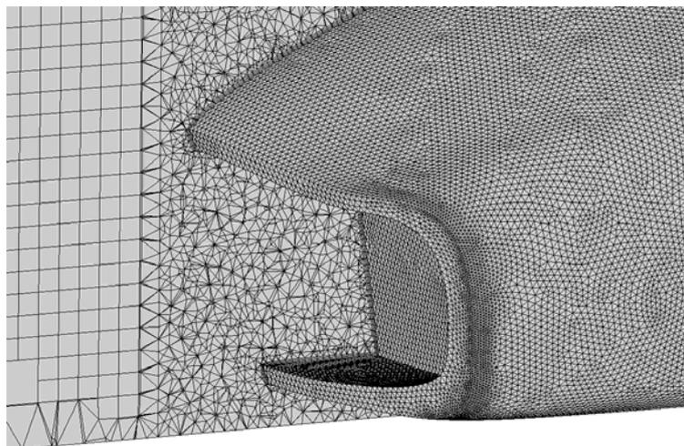
Figure 7 – The mesh at the front section of the car.
