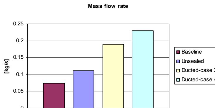
Figure 8 – The mass flow rate of the four cases.
