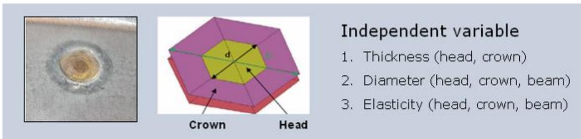
Figure 6 – Bolt spot weld model
