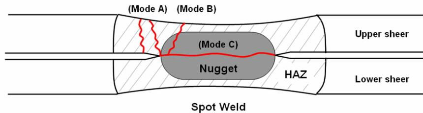
Figure 2 – Spot Weld Area
