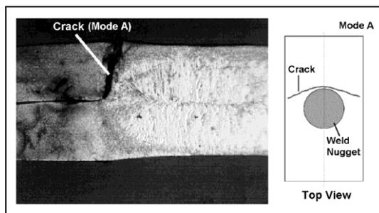
Figure 3 – sheet failure (Yi Gao[3])
