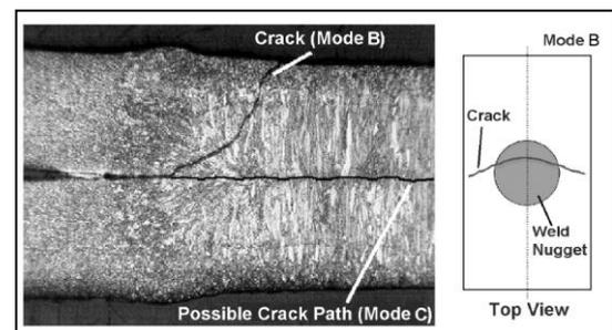
Figure 4 – nugget failure (Yi Gao[3])
