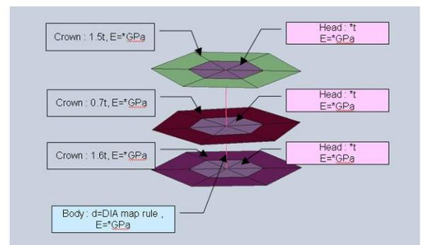
Figure 7 – variables of 3layer spot weld
