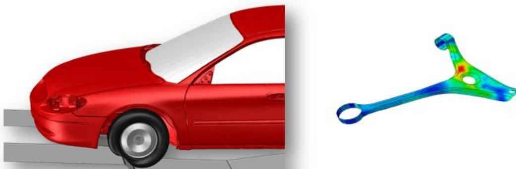
Figure 9: Pothole Impact simulation and the stress on the control arm
