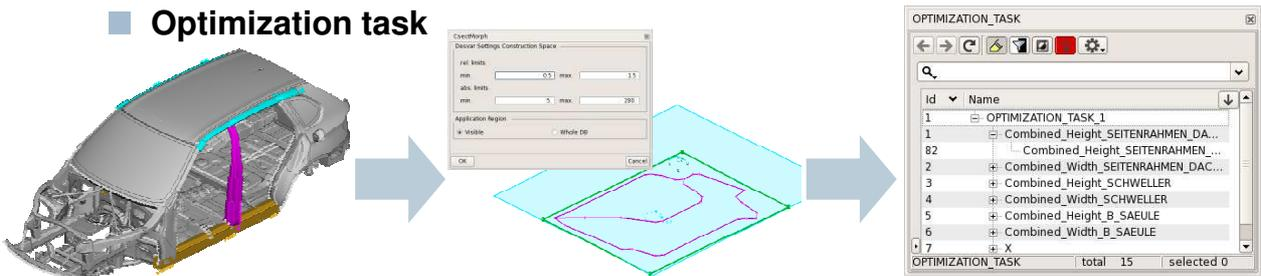
Optimization run with 200 mm extended wheel base model in order to reach original stiffnesses with combined construction space parameters of **roof carrier**, **b-pillar** and **rocker panel** as desvars
