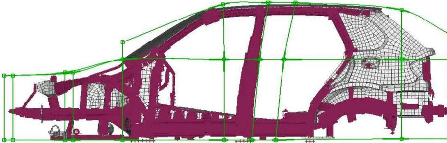
➔ Parameter study using Optimus, monitoring both global static and dynamic stiffness (eigenfrequencies) !
