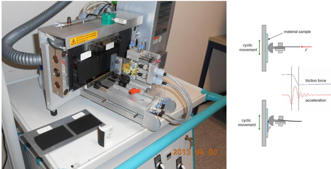
Figure 8 – Stick-slip test machine from Ziegler-Instruments GmbH used at VCC
