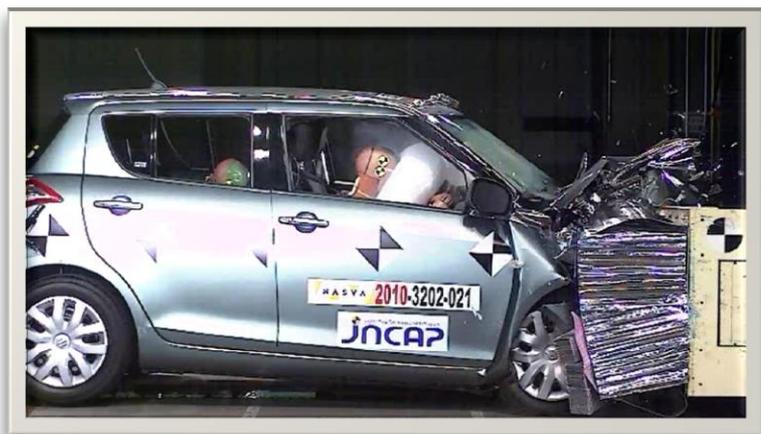
※ "Protection Against Electrical Shock After Collision Test" is also applied to Electric vehicles (EV-HEV). (Introduced from FY2011)
