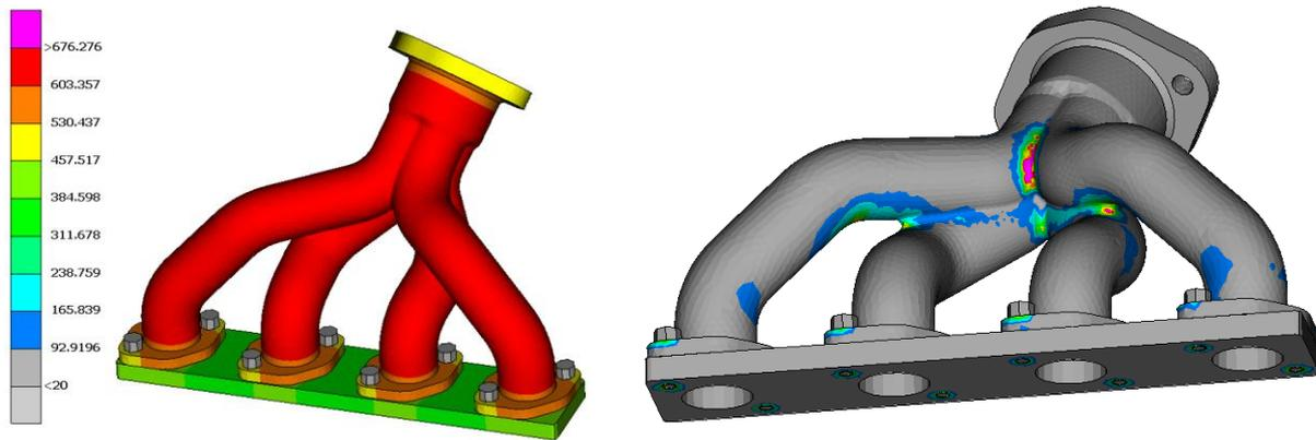
Figure 2 – Temperature field and resulting plastic strain distribution in the exhaust manifold
