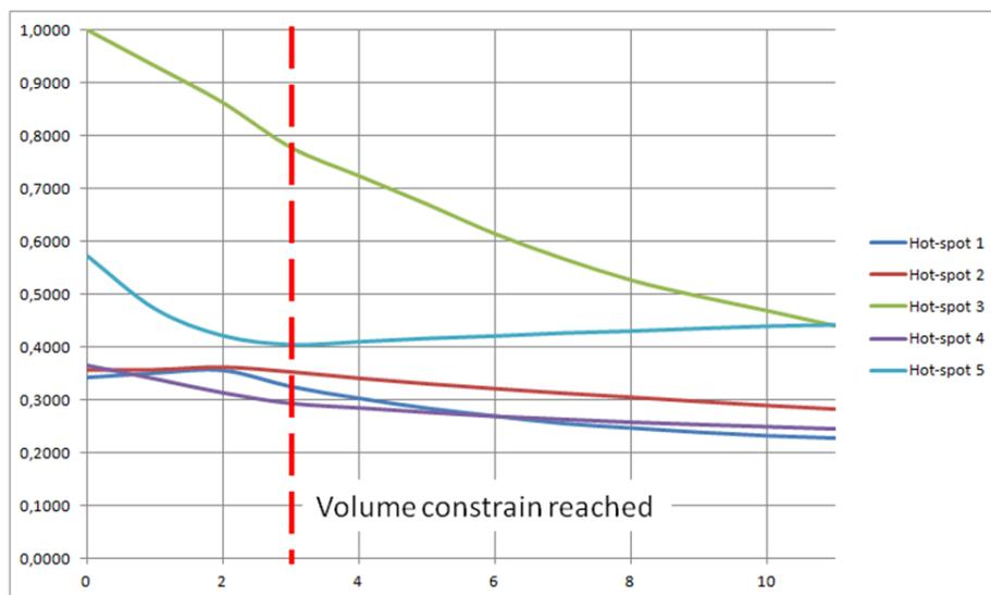
Figure 6 – Normalized plastic strain plots in the 5 critical regions over the iterations for a new combined optimization strategy
