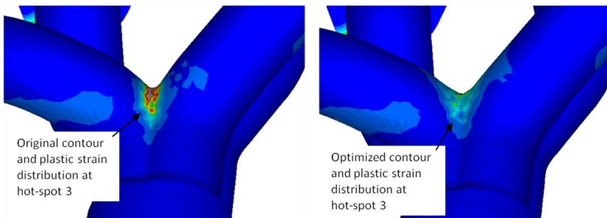
Figure 8 – Optimization of the geometry at maximum plastic strain location
