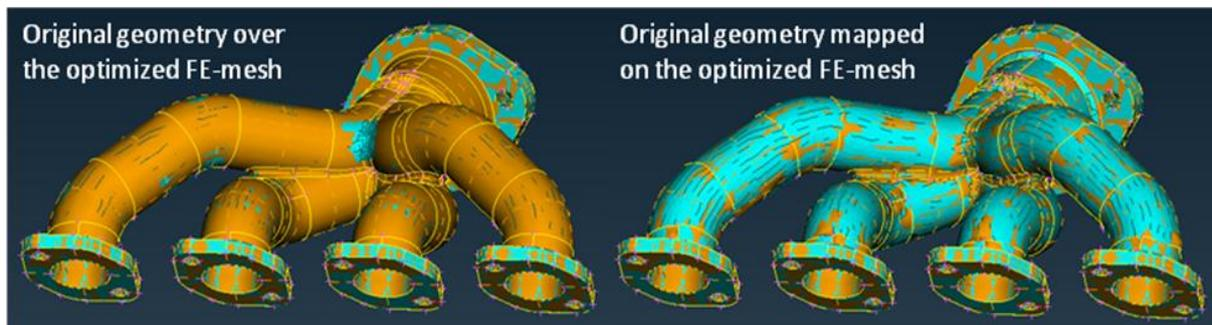
Figure 9 – Generating optimized geometry by mapping the original geometry to the FE-mesh of the optimized model
