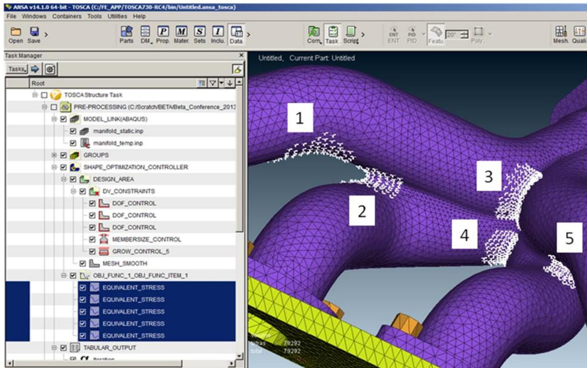
Figure 5 –TOSCA Structure shape optimization task in ANSA with highlighted hot-spots
