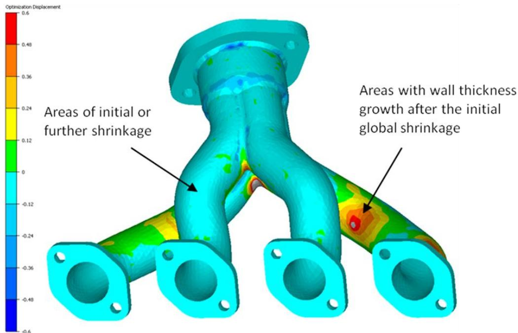
Figure 7 – Wall thickness change after the initial global shrinkage (iteration 4 to 11)
