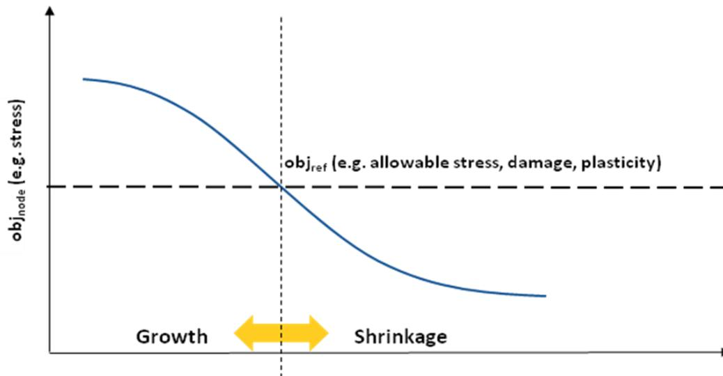
Figure 4 – Exemplary distribution of loading (objective) for an arbitrary part surface
