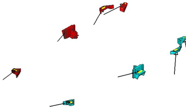
Figure 5: Study to evaluate relationship between load cases and design variables. One iteration of forces acting on battery pack fixing points
