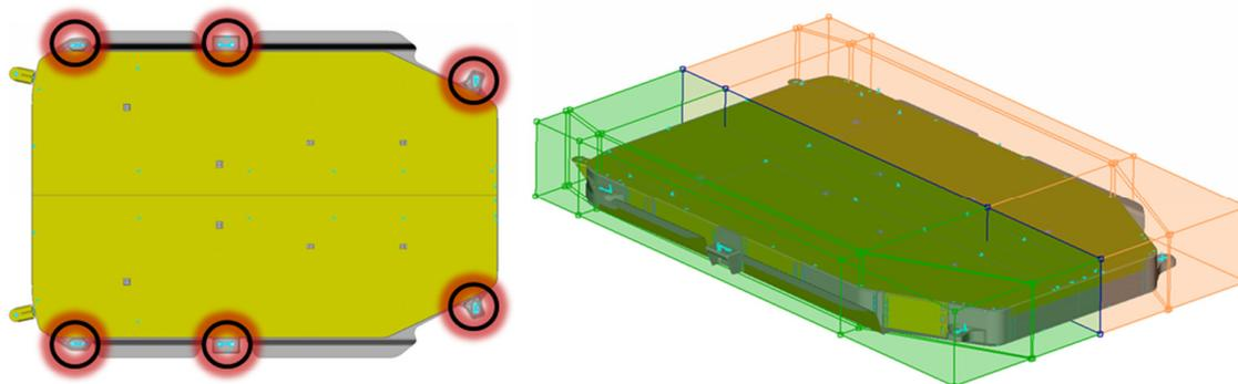
Figure 4 - Morphing conceptual parameterisation to develop optimal mountings (6 highlighted)
