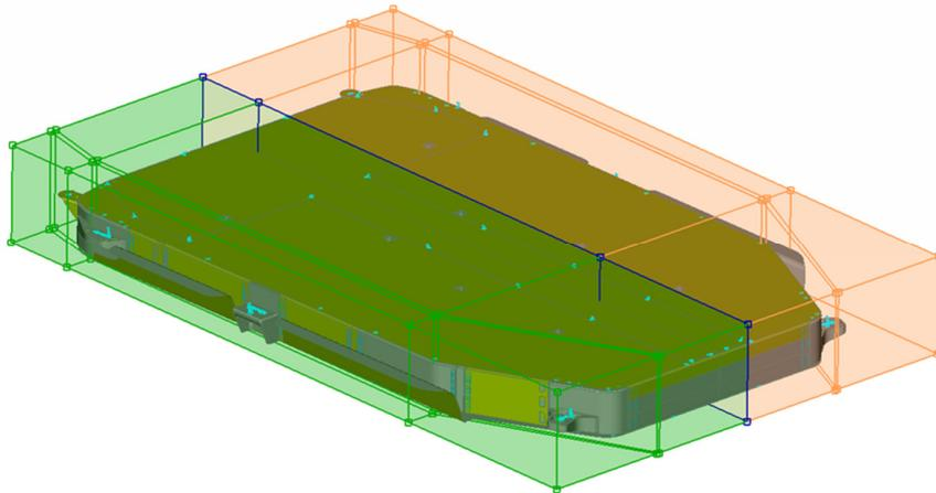
**Figure 2 – Basic Box Morphing Conceptual Parameterisation of a Battery Pack**
