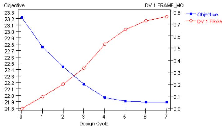
**Figure 3 - Optimisation Study using target values. In this graph it can be seen that most gains occurred by design cycle 5**
