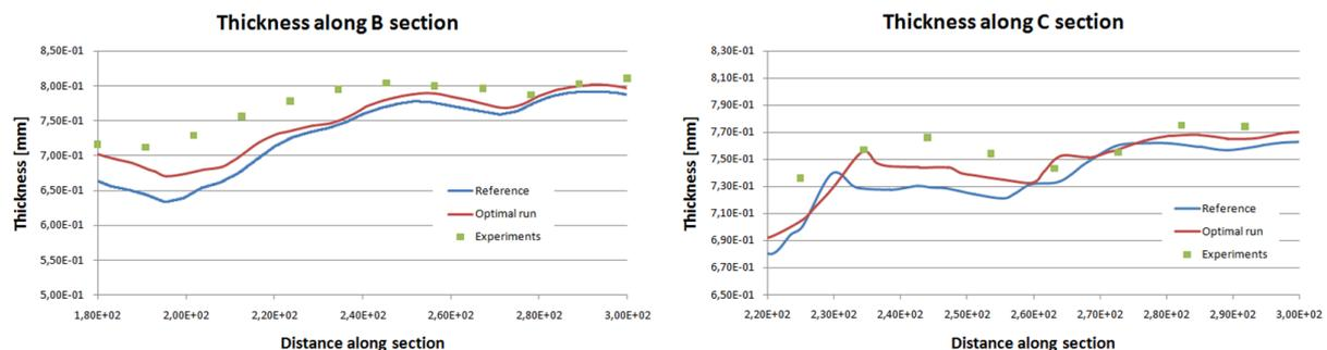
Fig. 15. Graphical comparison of thickness values along section B and C in multi–objective run.
