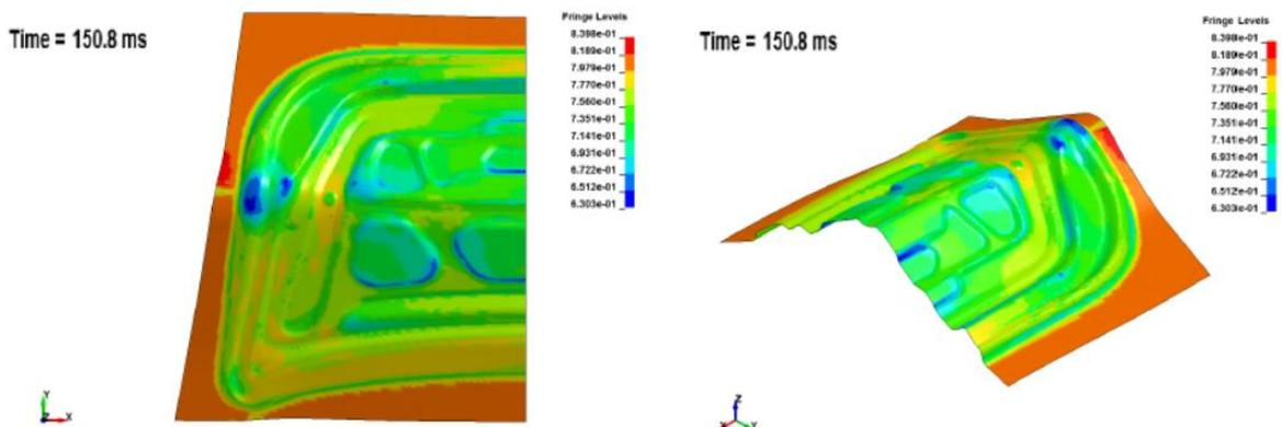
Fig. 11. Decklid thickness after forming
