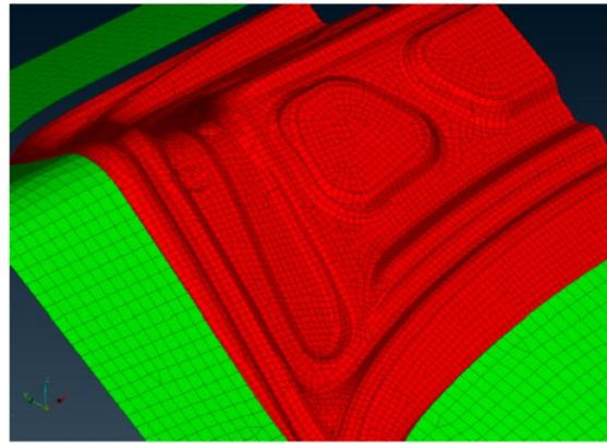
(b) Portions of the mesh of punch and binder, obtained with BEST algorithm.
