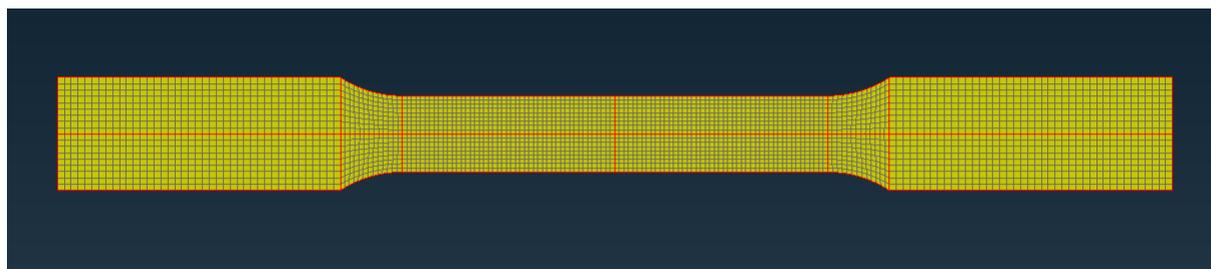
Fig. 2. Specimen mesh
