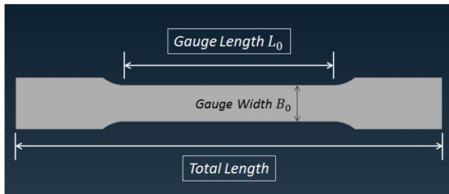
Fig. 1. Specimen dimensions
