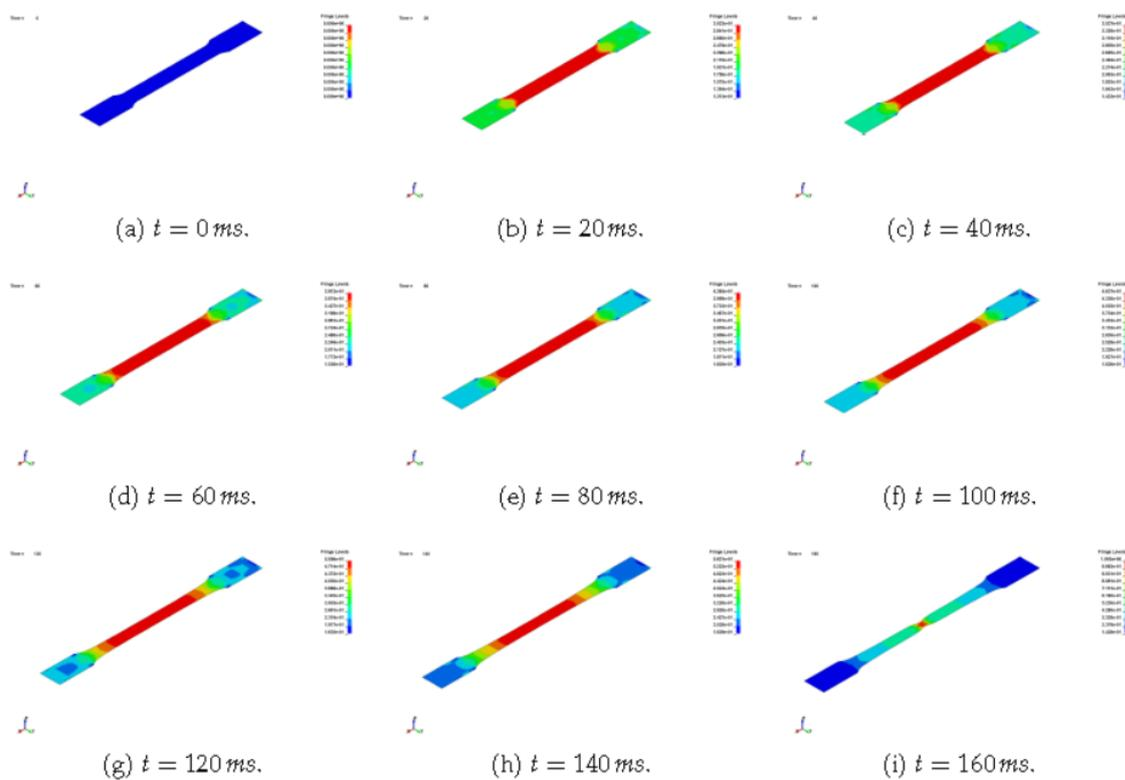
Fig. 5. Von Mises Stress on the specimen during tensile test
