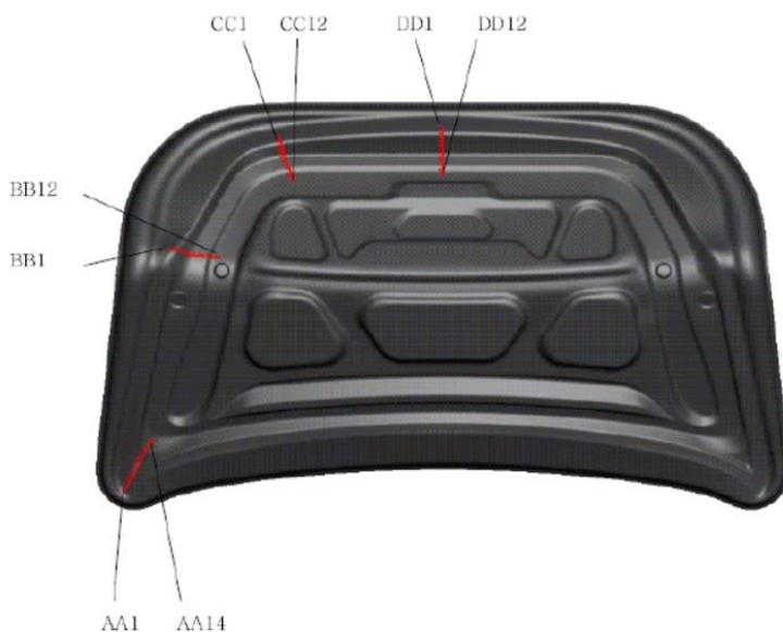
Fig. 13. Sections for which benchmark documentation provides thickness data
