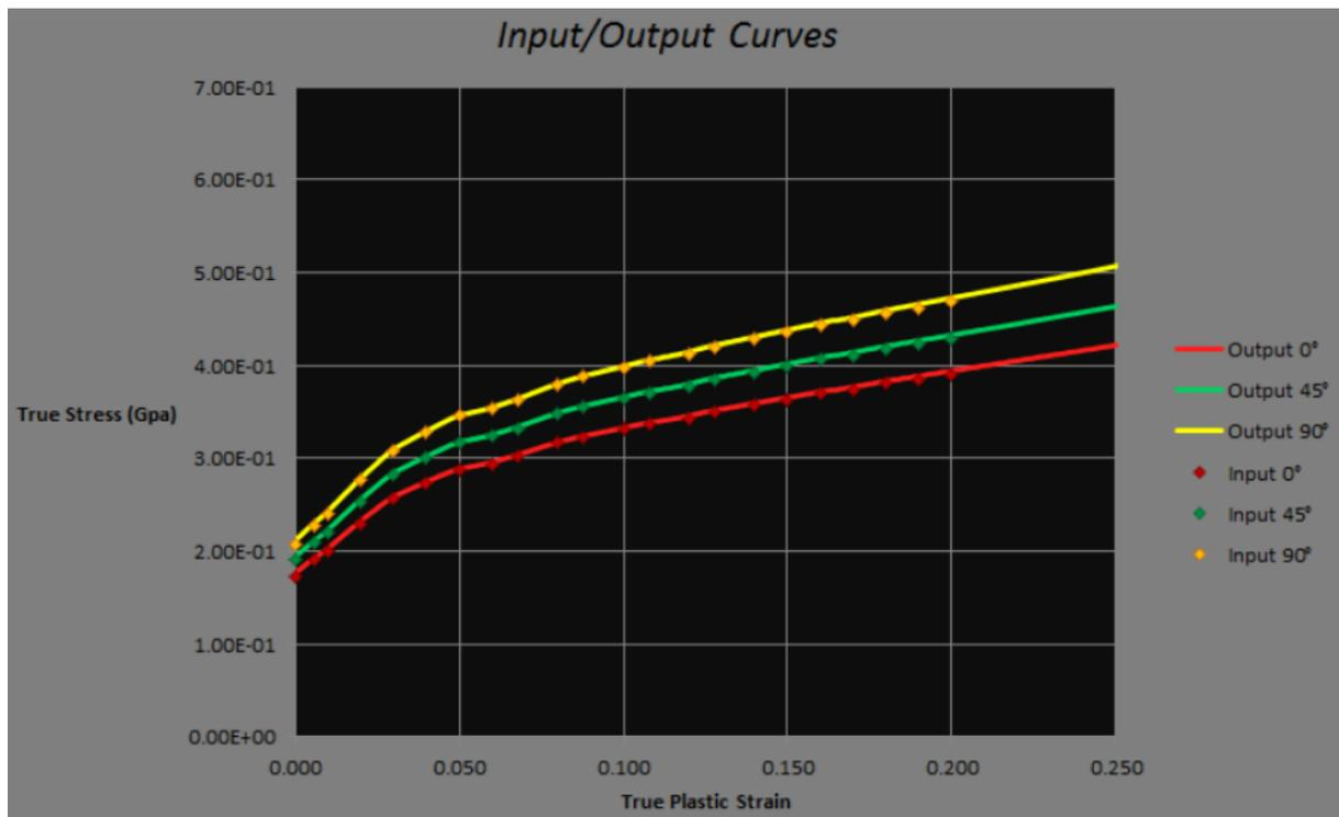
Fig. 4. True Stress vs. True Plastic Strain Input/Output Curves
