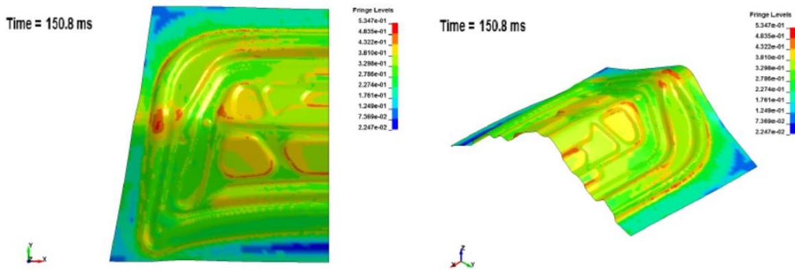
(c) Top view of the blank with Von Mises contours. (d) Isometric view of the blank with Von Mises contours.
