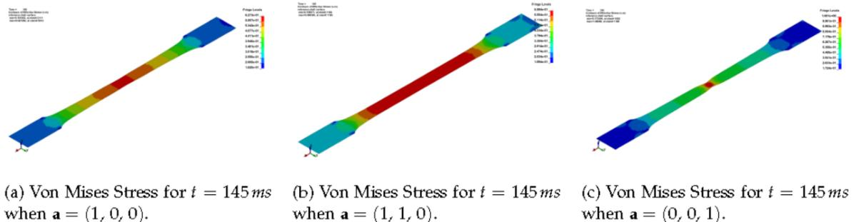
Fig. 6. Different specimen deformations due to different rolling directions
