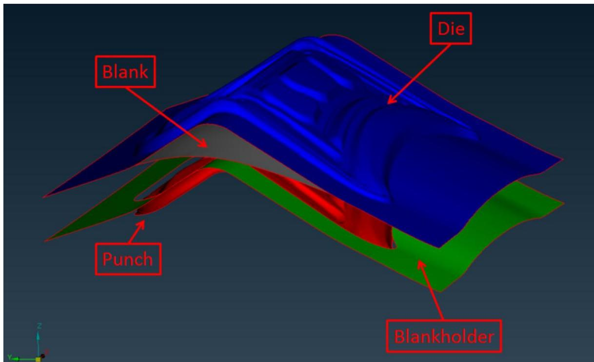
Fig. 7. Tools arrangement with the sheet metal
