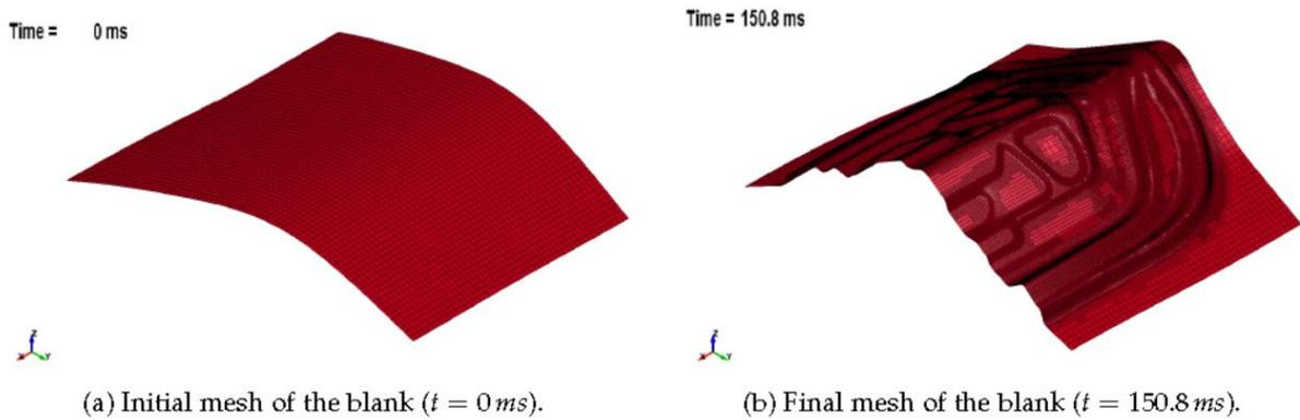
Fig. 10. Adaptivity on the blank mesh: while the border is unchanged, the internal part is extremely thicker
