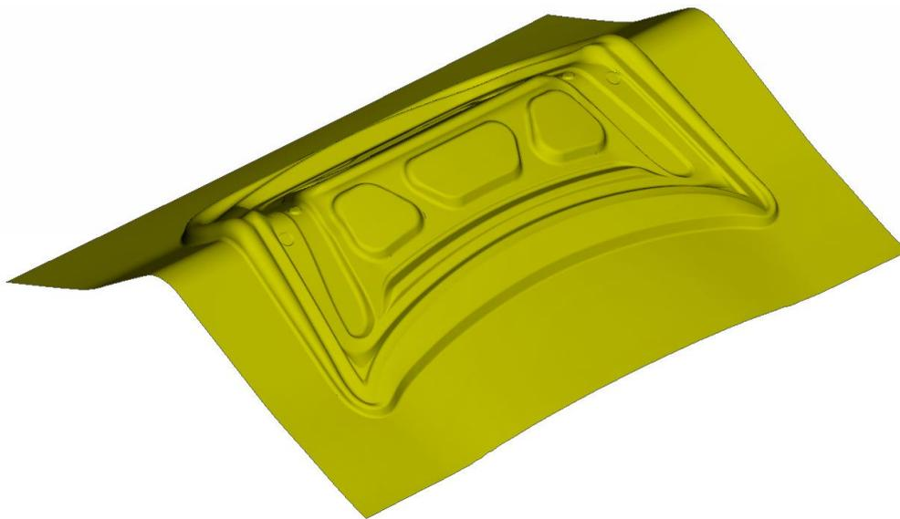
Figure 9 – Output of 'Offset punch and binder from die surfaces' option
