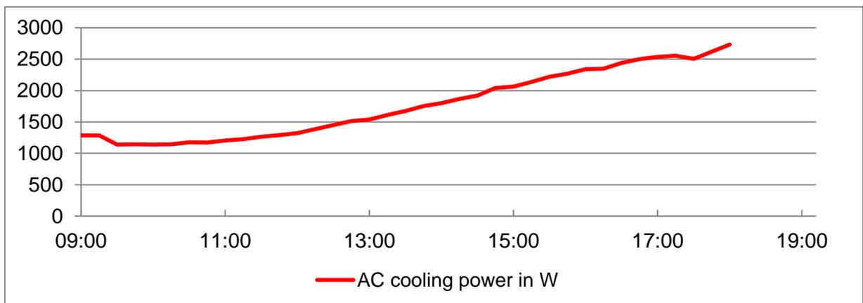
Figure 21: AC cooling power for blind down
