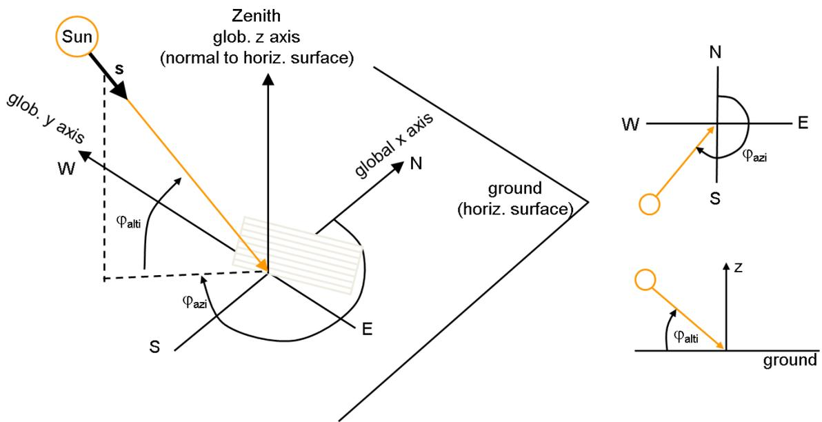
Figure 3: Definition of solar azimuth and altitude
