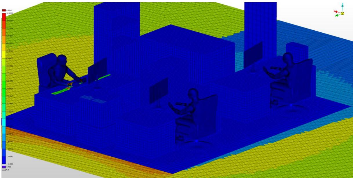
Figure 15: Solar irradiation at 18:00, blind closed. Almost no sunlight reaches the office in this case.
