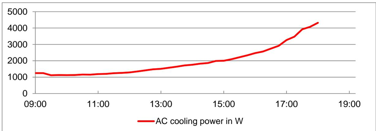
Figure 18: AC cooling power with blind up and AC on.
