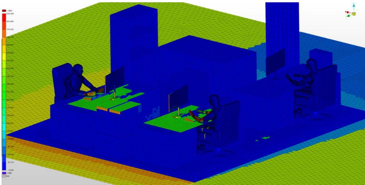
Figure 12: Solar irradiation at 18:00. Bob in the middle receives direct sunlight on his lower arms, resulting in off-the-scale PMV values.
