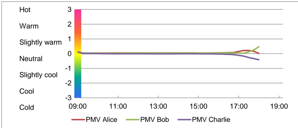
Figure 17: PMV values for all three occupants with blind open
