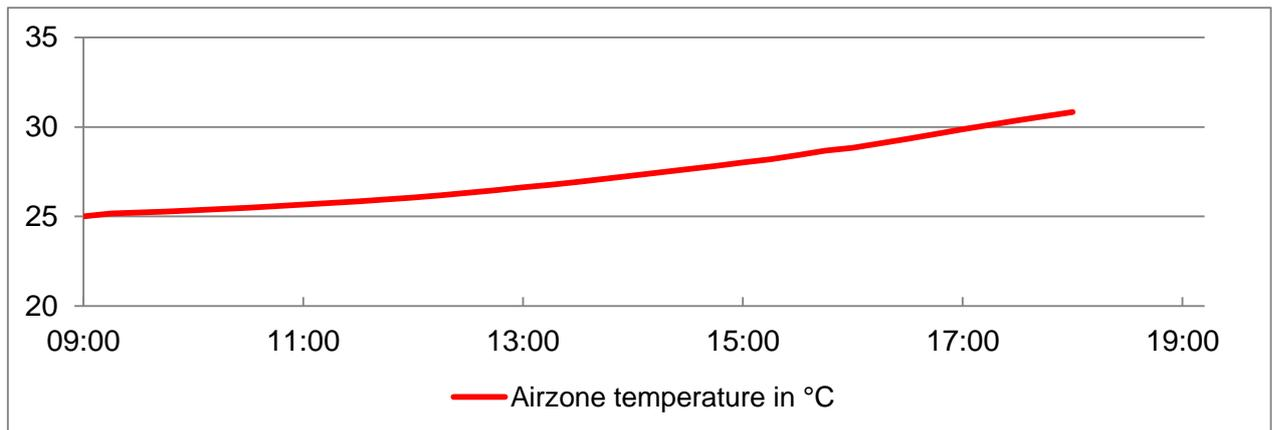
Figure 10: Average air temperature within the office container
