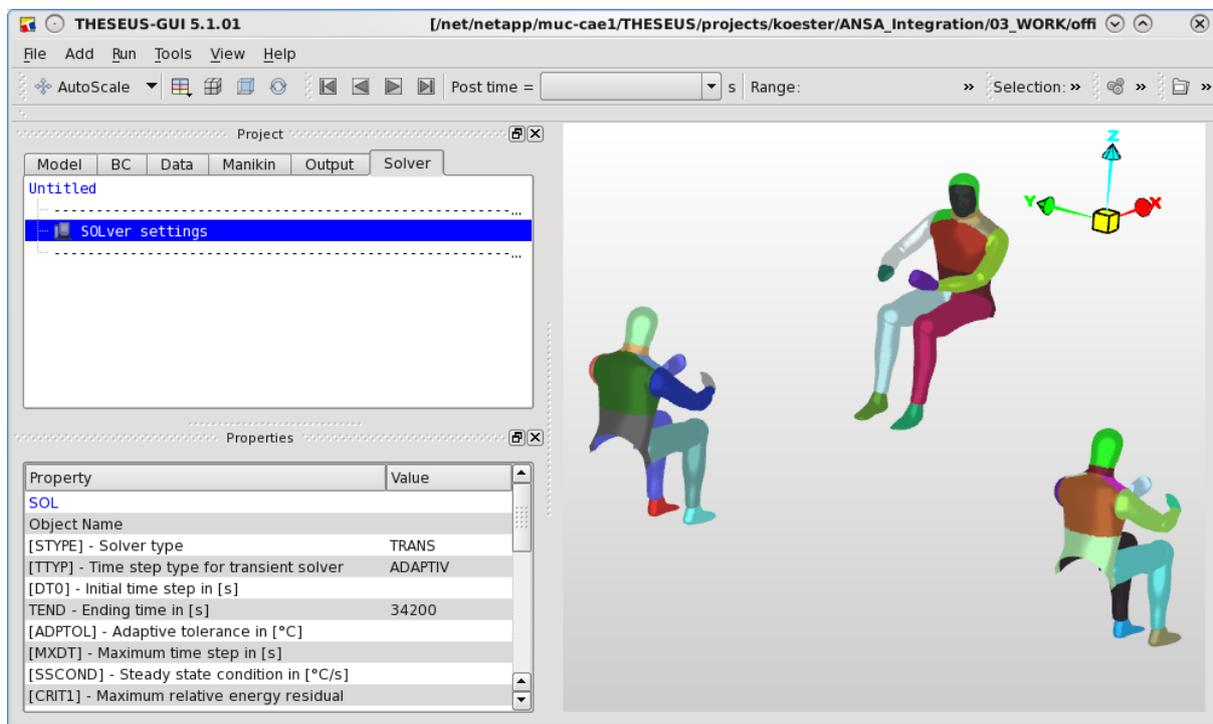
Figure 9: Case components defined within the THESEUS-FE GUI: manikins, post-processing, and solver definitions
