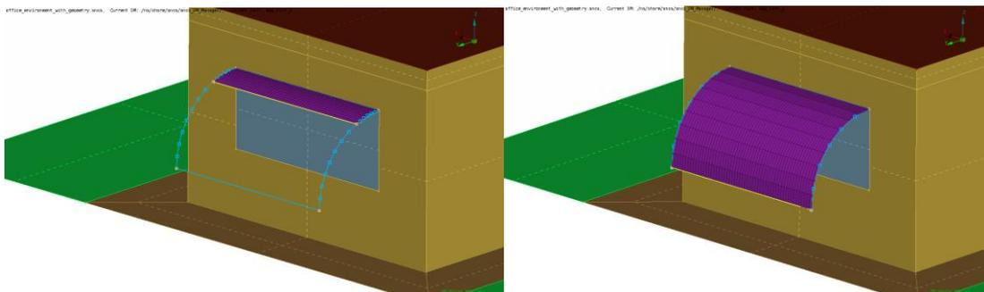
Figure 8: Parametrized movement of the window blind
