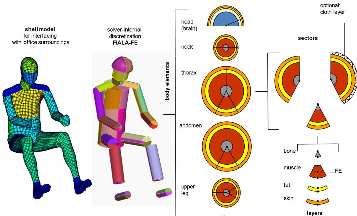
Figure 6: Principles of the thermal manikin model FIALA-FE
