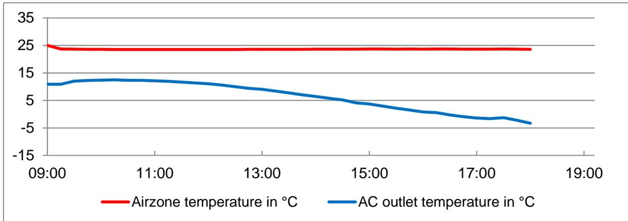
Figure 19: Office and AC outlet temperature with blind down and AC on
