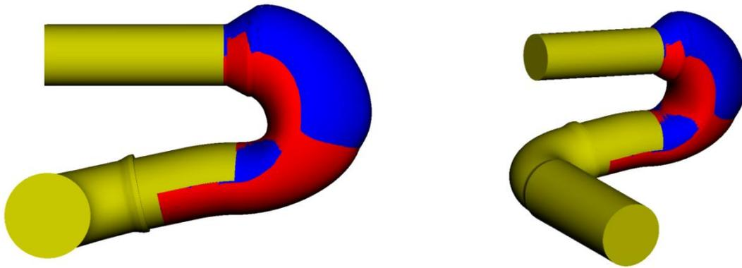
Figure 4 – Differences between the designs where red is Baseline design and blue is optimized design. Yellow color means no difference between the designs.
