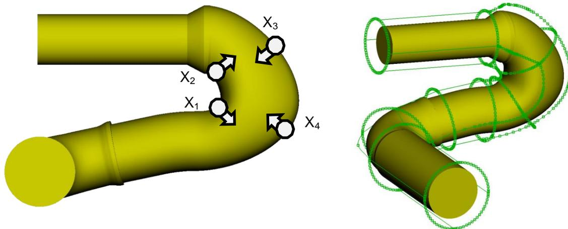
Figure 3 – Design variable locations and surrounding morphing boxes. The arrows display the positive direction for each design variable.
