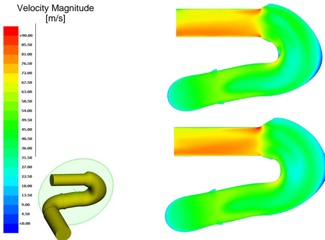
Figure 5 – Velocity magnitude in cross-section plane of turbo pipe for baseline design (at top) and optimized design (at bottom)
