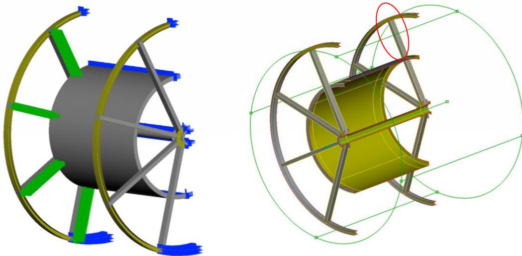
Figure 7 – Model of the cable drum highlighting boundary conditions and loads on the spokes (left) and model showing the morphing box and the purpose of the extend operation (right).
