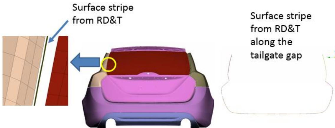
Figure 11 – Importing the surface stripe in ANSA for the E-line calculation.
