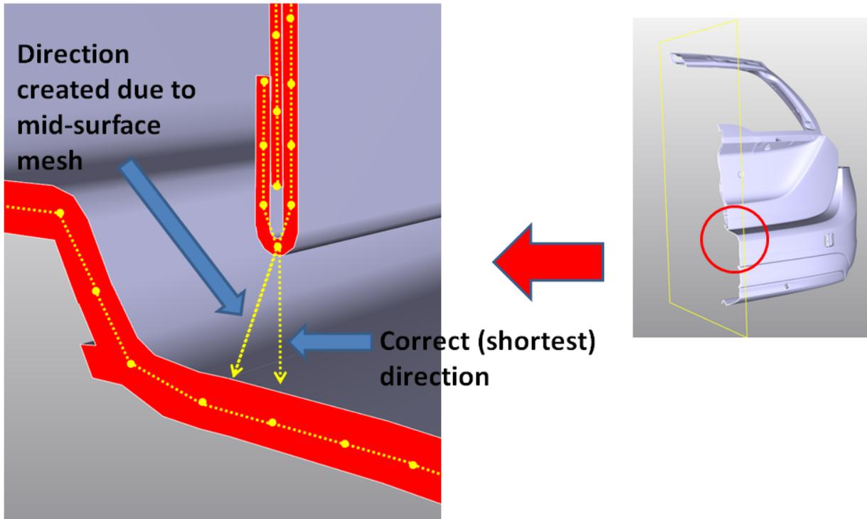
Figure 13 – CBUSH orientation due to mesh (A) and surface stripe (B) based E-line.
