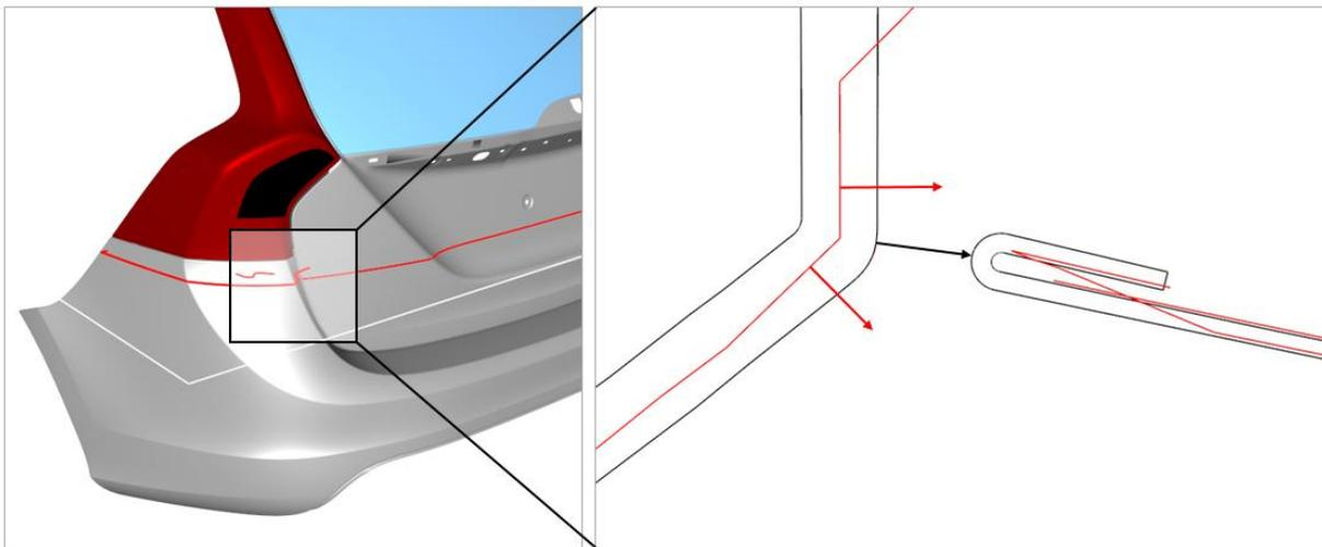
Figure 8 – Different possible evaluation directions due to different mesh qualities.
