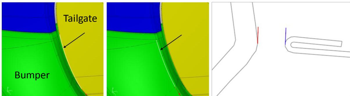
Figure 10 – (A) Surface stripes based on tailgate support line. (B) Surface stripes based on bumper support line (C) Section with the two parallel surface stripes.
