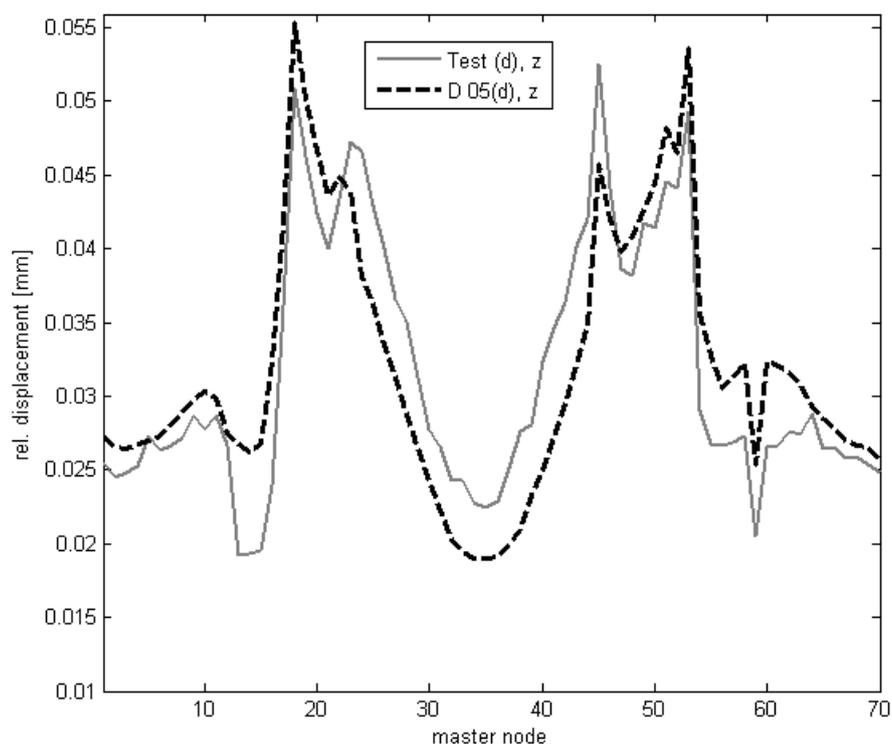
Figure 7 – Relative displacement in local z direction for test and simulation (setup 1) [4].
