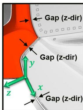
Figure 5 – E-line local directions, 'z' is the gap direction, 'y' is perpendicular and 'x' is along the line [4].
