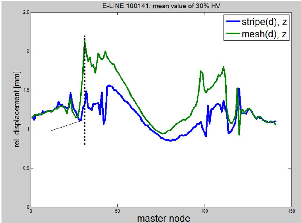
Figure 14 – Relative displacement in local z direction for Mesh based and surface stripe E-lines.
