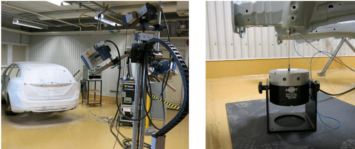
Figure 2 – 3D laser cameras pointing to the rear end (A), shaker location in the front end (B) [4].
