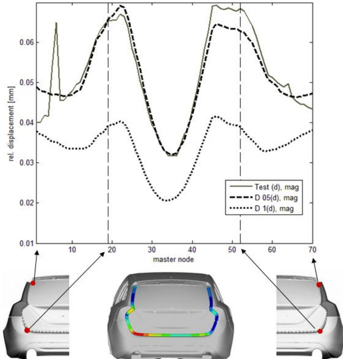
Figure 6 – Comparing relative displacement between test and simulation. The relative displacement plot starts at the upper left corner and ends at the upper right [4].
