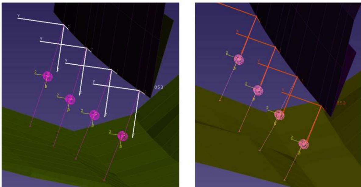
Figure 12 – CBUSH orientation due to mesh (A) and surface stripe (B) based E-line.
