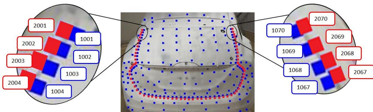
Figure 3 – Defined measurement points on the test object – point pairs along the gap [4].
