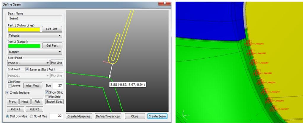
Figure 9 – (A) Seam creation interface. (B) Defined measurements along the seam.
