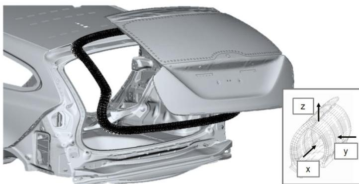
Figure 4 – Sealing represented by spring elements [4].
