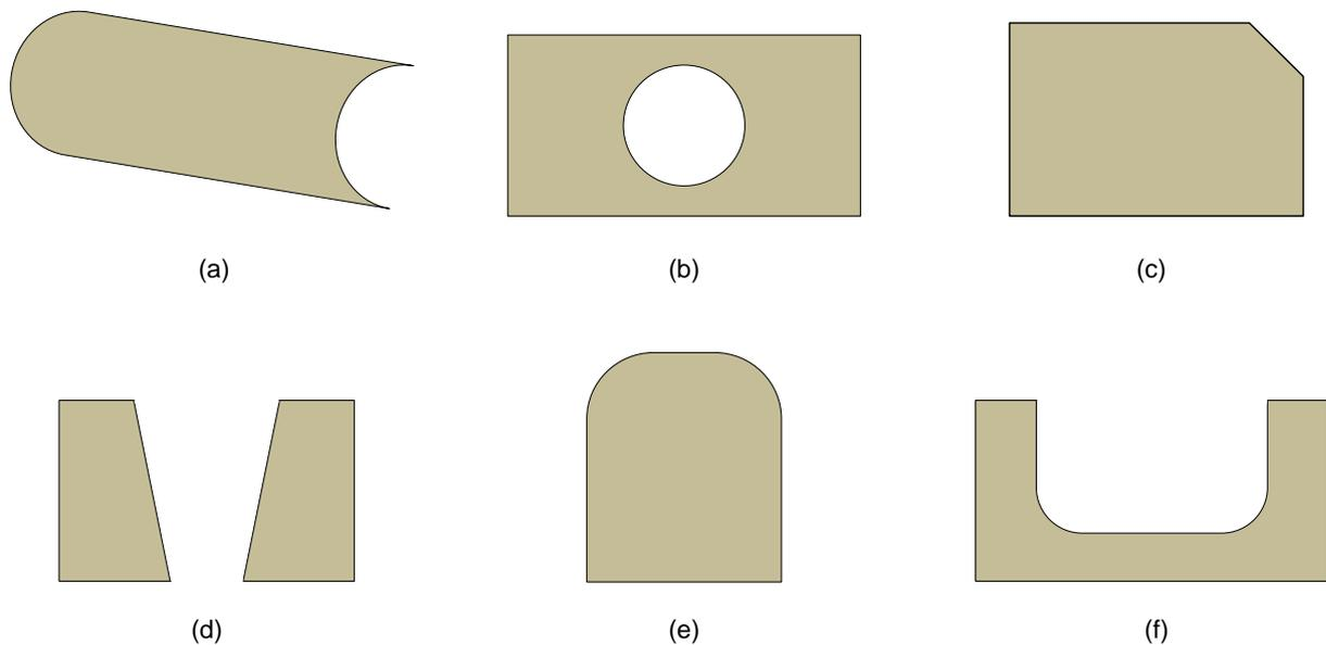
Figure 2 – Face shape and feature examples. (a) fillet, (b) hole, (c) chamfer, (d) tapered holes, (e) rib, (f) groove
