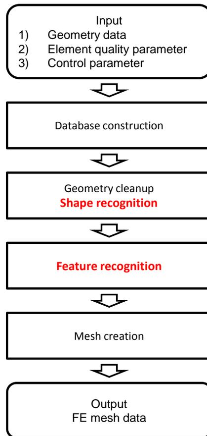
Figure 1 – Main procedures of automatic mesh generating system using ANSA script.
