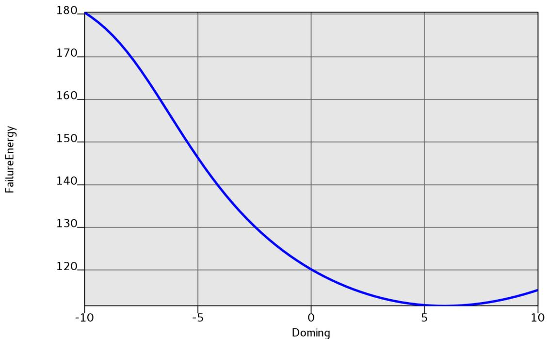
Figure 8 – Effect of Doming on Energy to Failure
