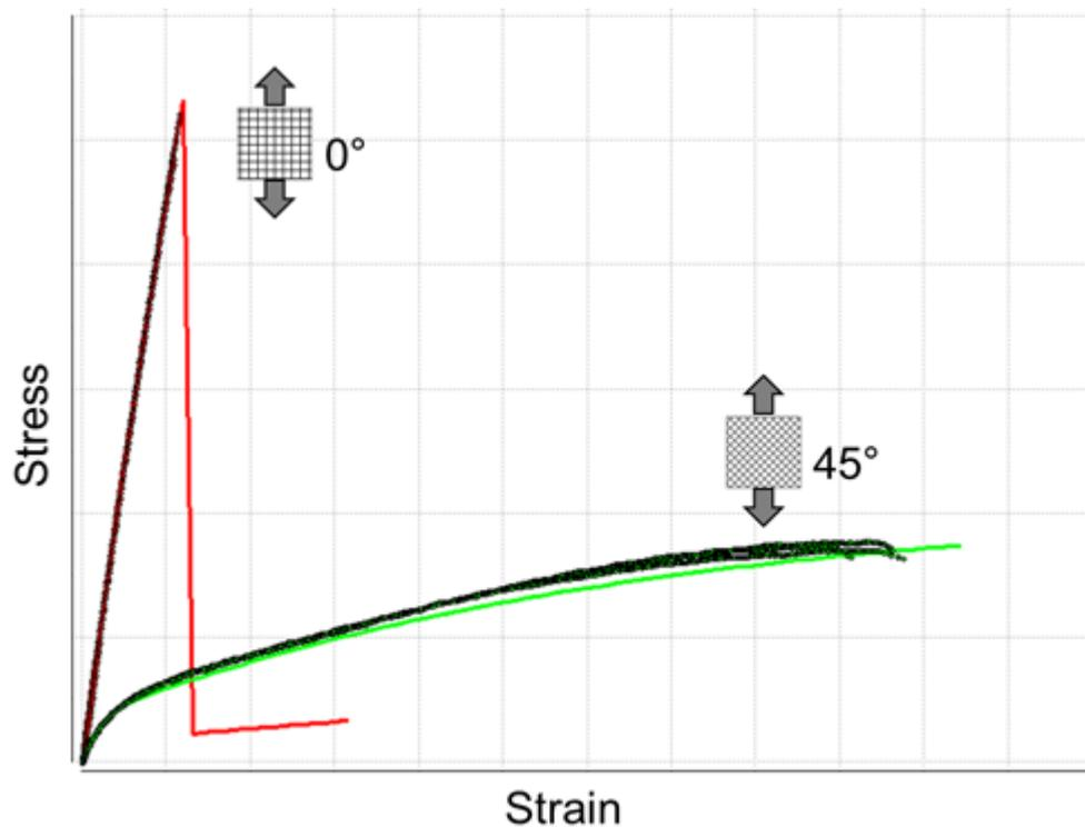
Figure 1 – Effect of woven laminate fiber orientation on stress-strain curve. (5)
