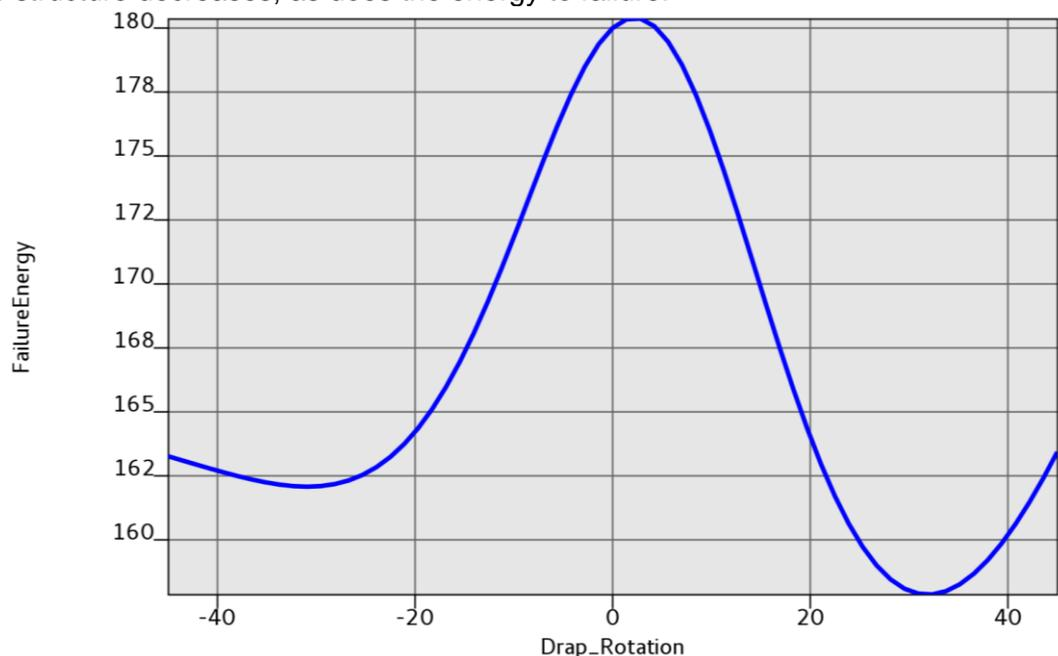
Figure 7 – Effect of Draping Angle on Energy to Failure.
