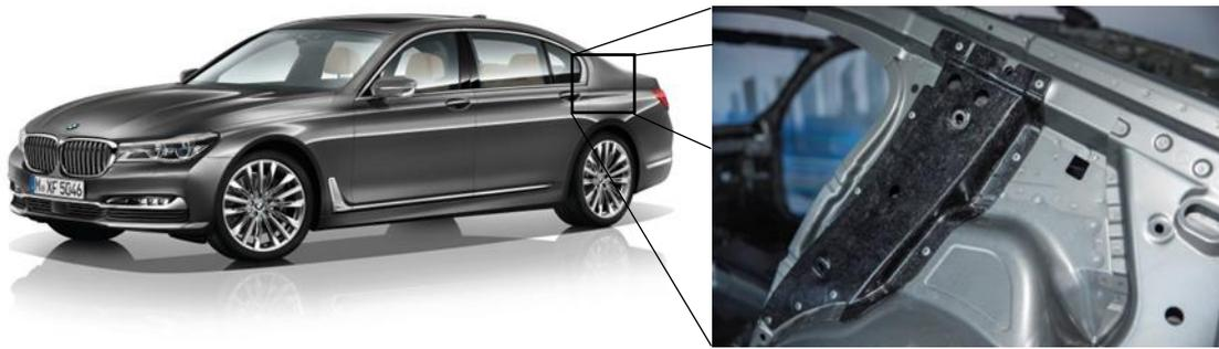
Figure 1 – Reinforcement of the C-pillar (right side) made of Carbon Fiber Sheet molding compound (CF-SMC) in the body structure of the BMW 7 (G11/G12) series (1).
