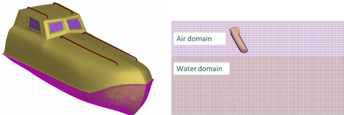
Figure 2 – Shell mesh on boat surface (left) and ALE interaction of the fluid domains with the solid object
