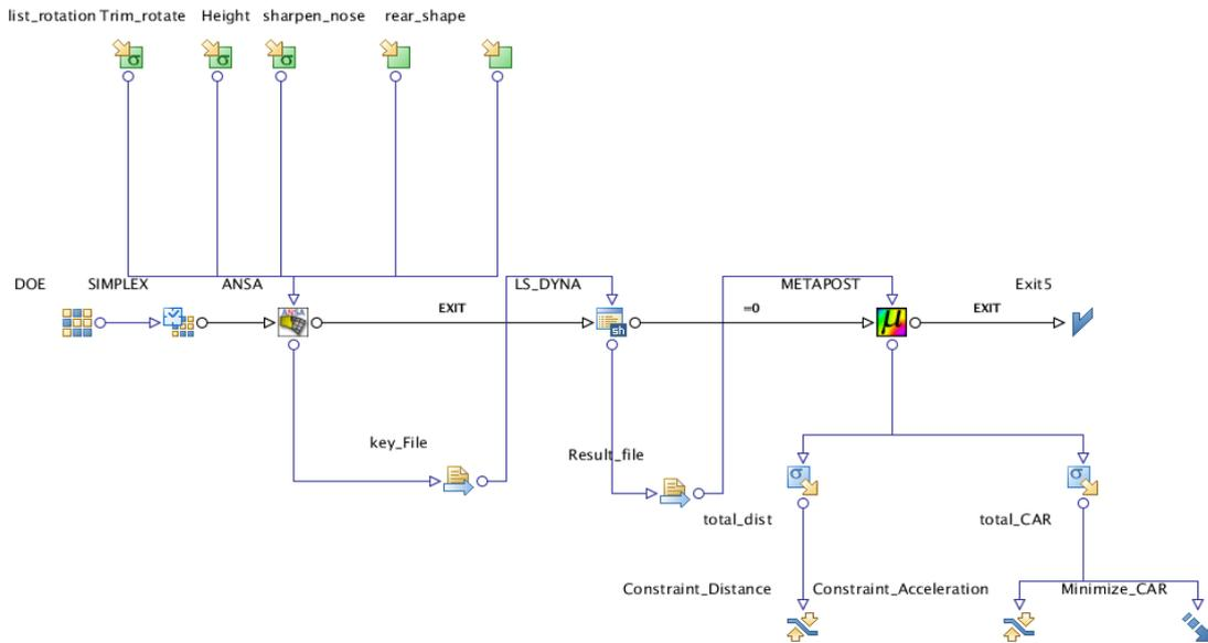
Figure 6- modeFRONTIER workflow for the lifeboat reliability optimization
