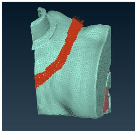
Figure 8 The distributed load on the neck.
