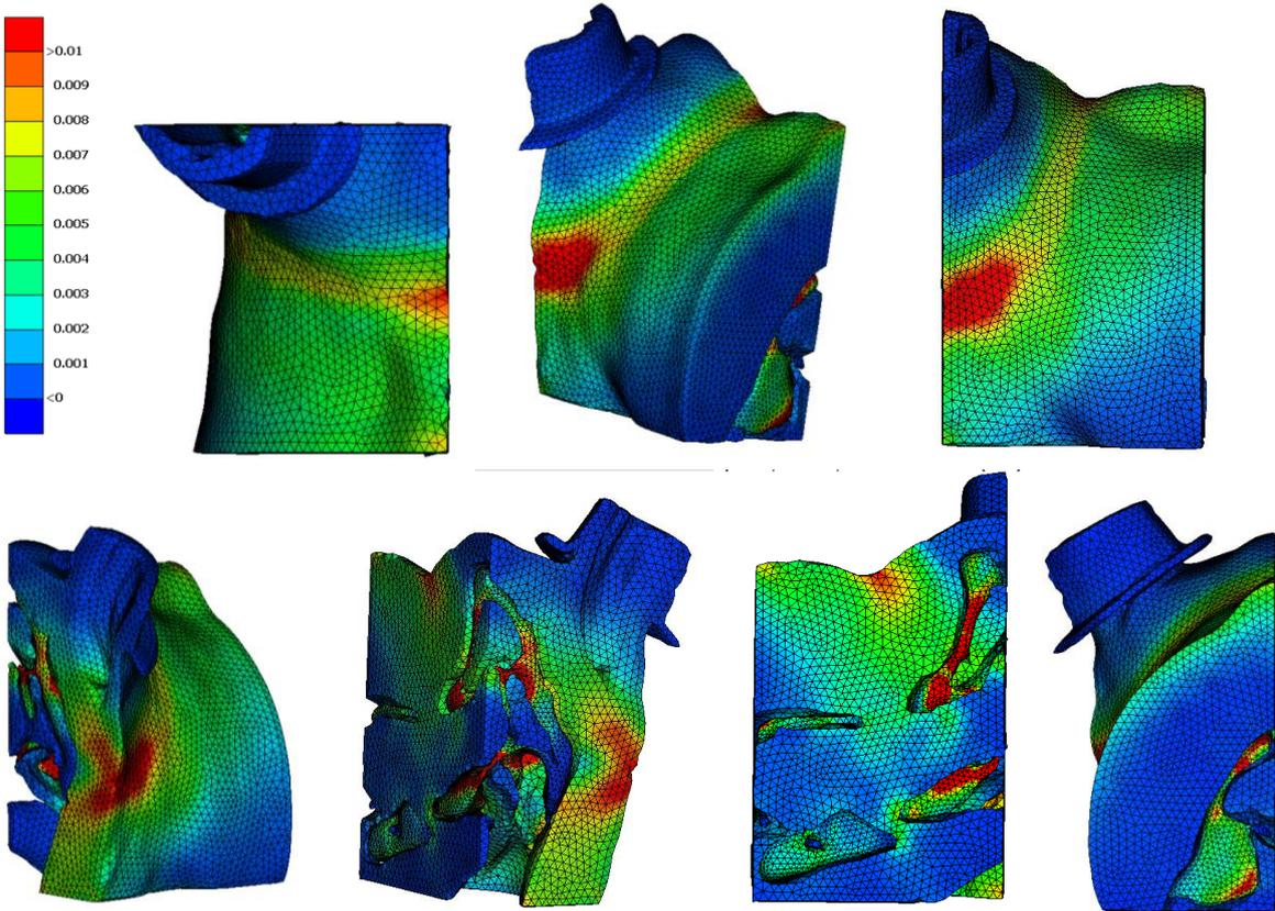
**Figure 9** The von Mises stress distribution for Yeoh material model. The unit of the colorbar is MPa.
