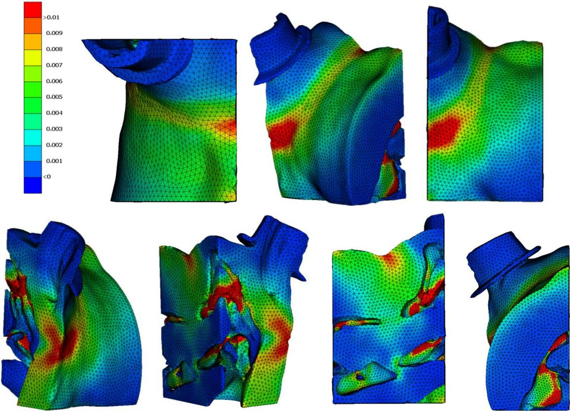
**Figure 10** The von Mises stress distribution for Ogden material model. The unit of the colourbar is MPa.
