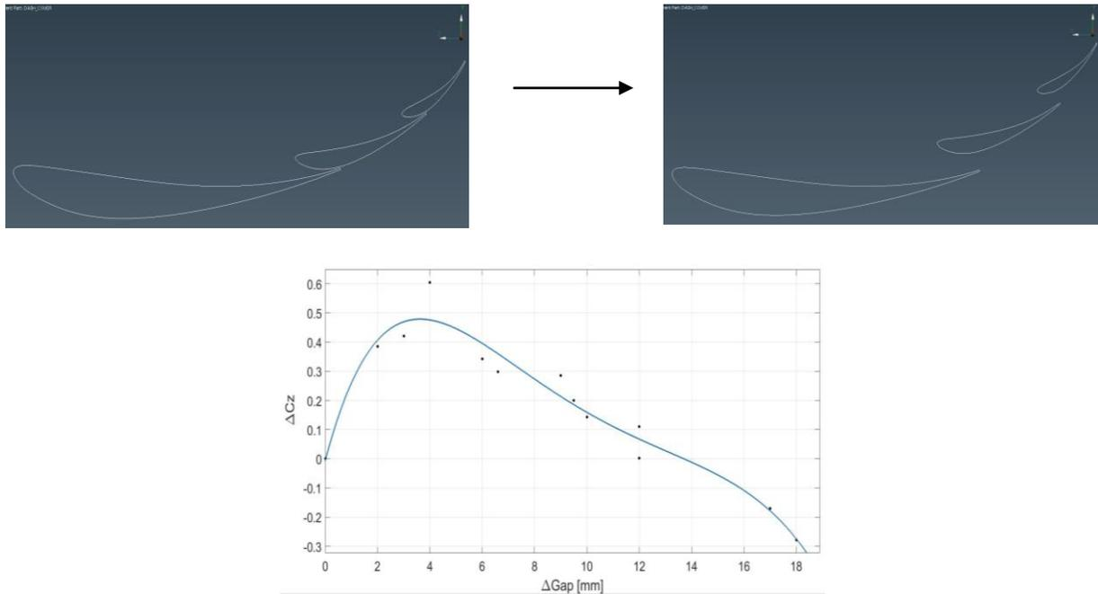
Figure 4: Downforce variations with increasing slot gap
