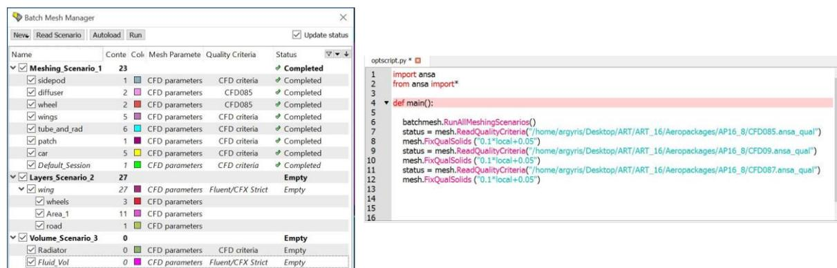
Figure 1: Batch Mesh Tool and scripting for parallel simulation on a cluster
