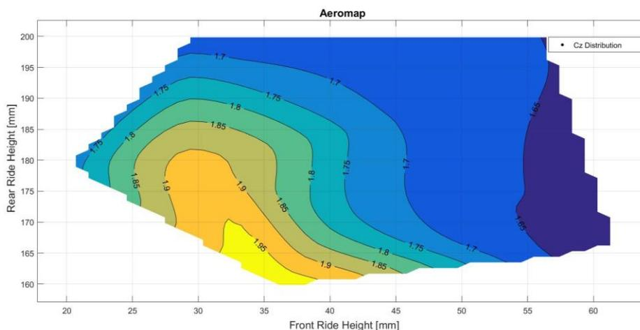
Figure 5: Downforce coefficients for different front and rear ride heights
