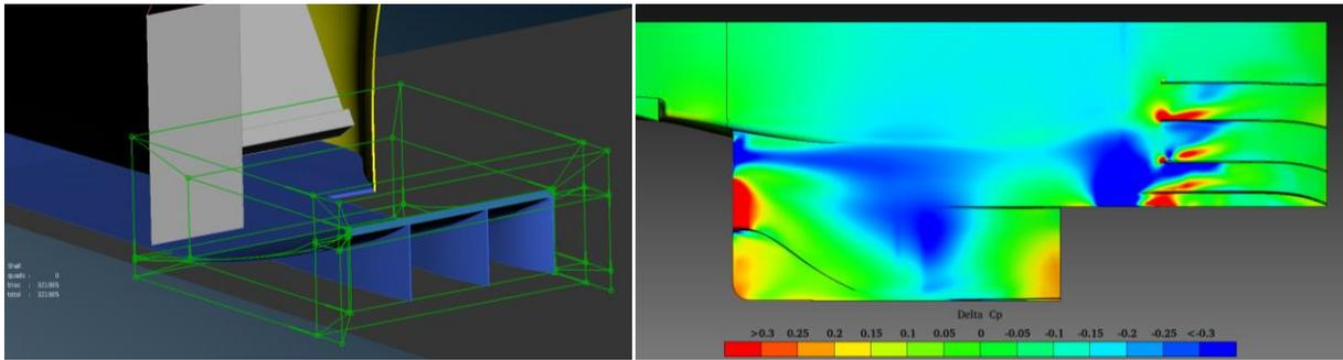
Figure 3: Diffuser's morphing boxes and Pressure Coefficient differences between initial and final diffuser design
