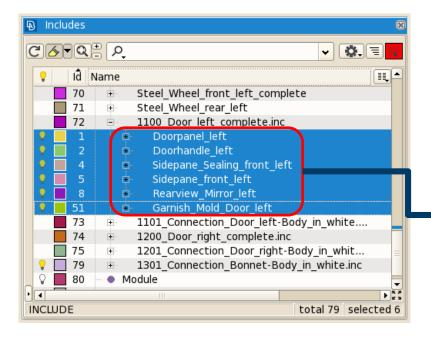
Make sure, that all related entities are moved to the MODULE, like nodes, elements, properties,...., by using subcontainer rules.
