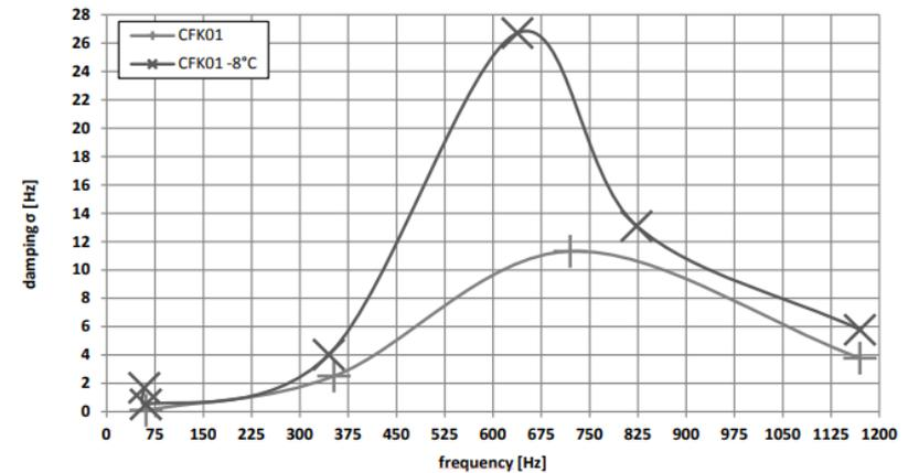
Modal Damping ratio v/s Resonance Frequency of CFRP at 23C and -8C.
