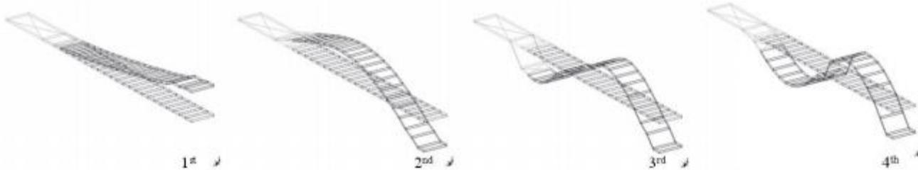
Mode Shapes of CFRP Leaf Spring
