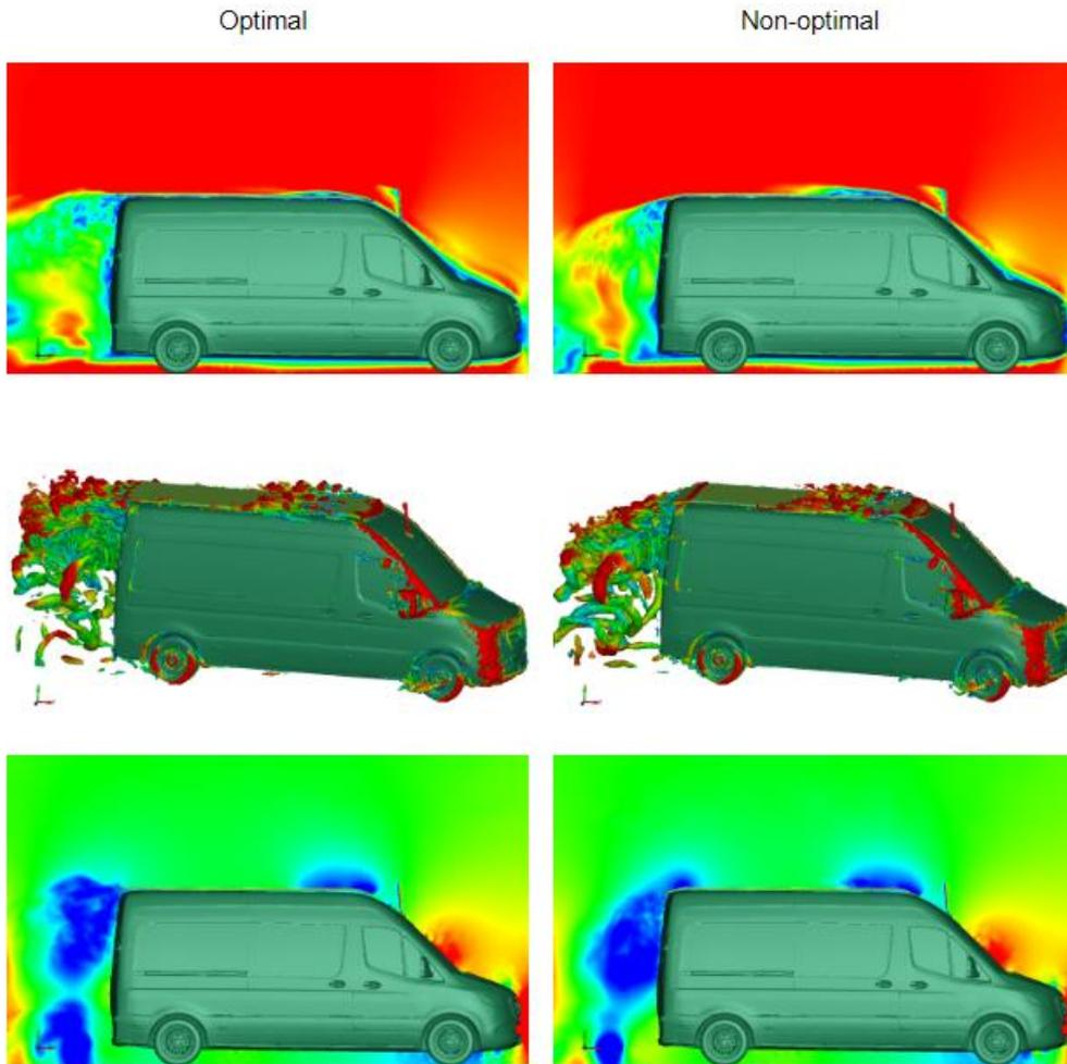
Figure 7 – CFD results comparison between the optimal result and a non-optimal iteration showing the flow features near the roof racks and behind the vehicle. Top: time-averaged velocity on section plane. Middle: Q criterium coloured by the velocity field. Bottom: time-averaged pressure field.
