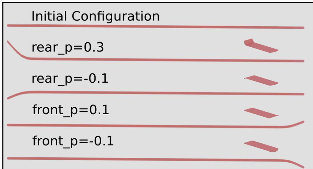
Figure 2 –Parameters used in the optimization loop and the extreme roof racks configurations.
