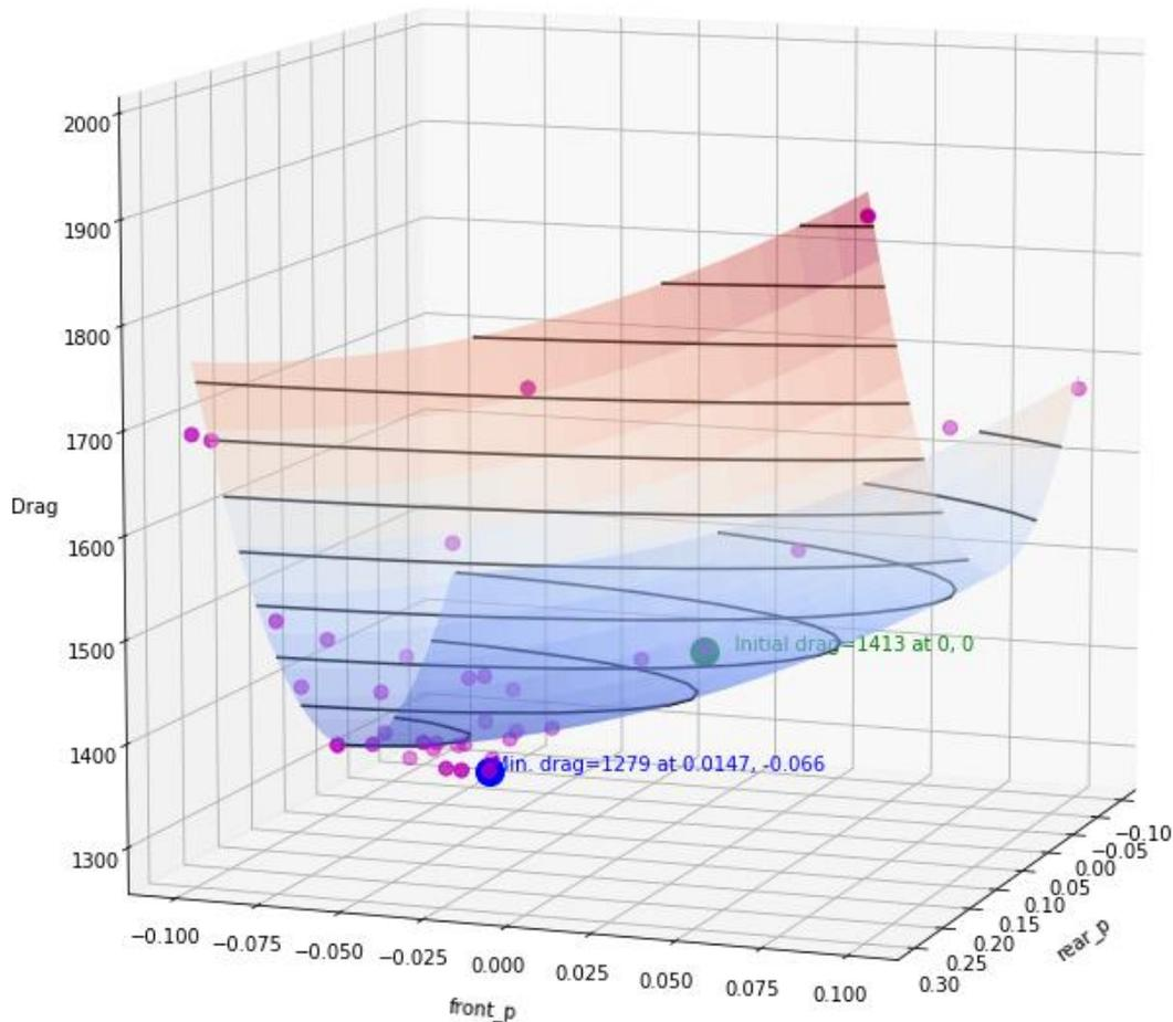
Figure 6 – Optimization results after 10 iterations of LS-OPT. Blue colour shows the minimum value while green shows the initial configuration.
