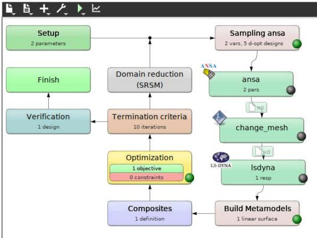
Figure 4 –LS-OPT flow chart for the optimization metamodel “Sequential with Domain Reduction”.
