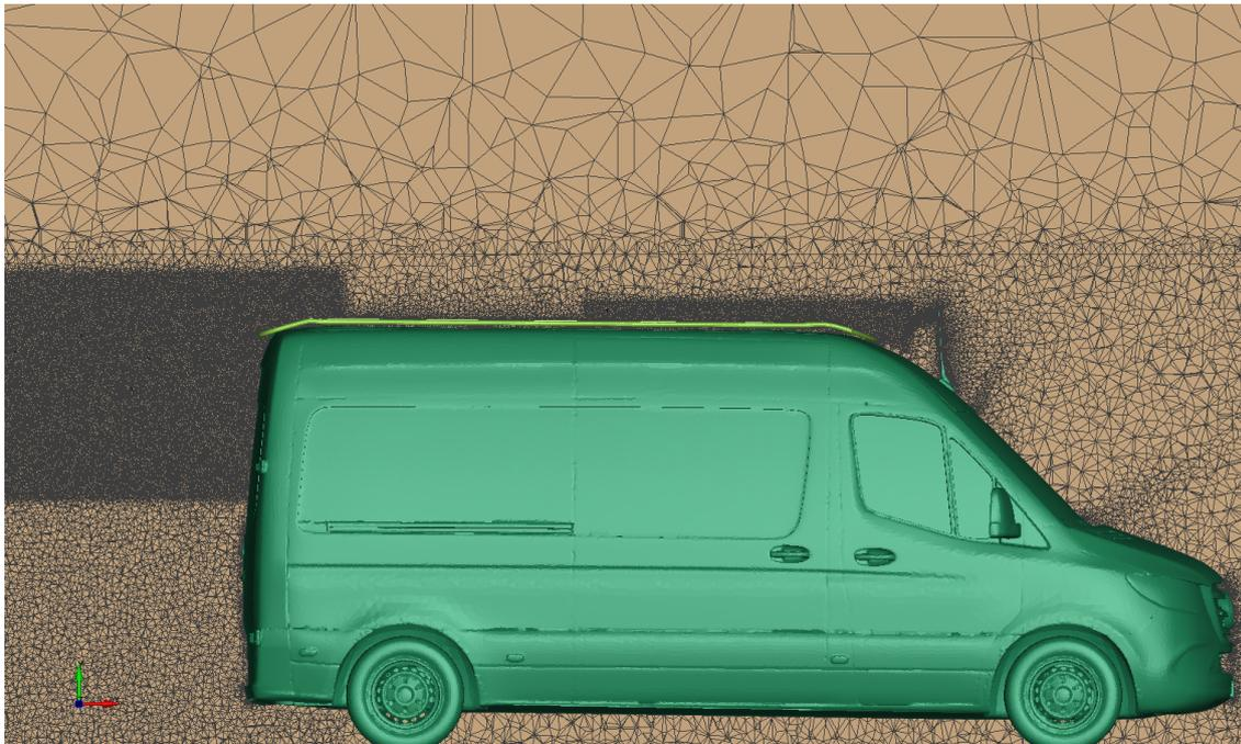
Figure 5 –Section cut of the volume mesh showing the refinement regions at the leading and trailing edges of the roof racks.
