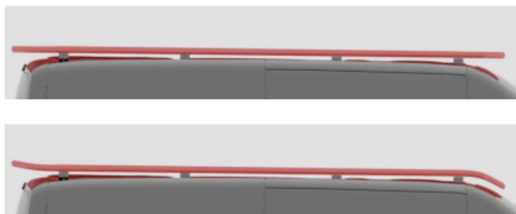
Figure 8 – Comparison between the initial and the optimal roof racks configuration.
