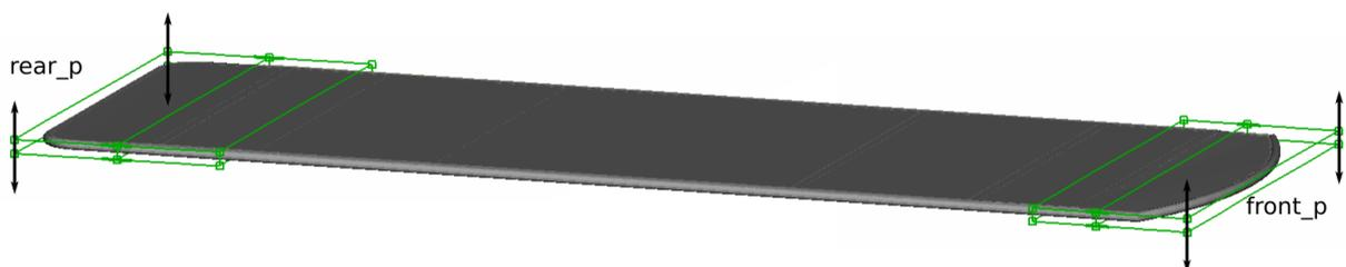
Figure 3 – Rear and front morphing boxes defined in ANSA to modify the geometry using parameters  $rear\_p$  and  $front\_p$ .
