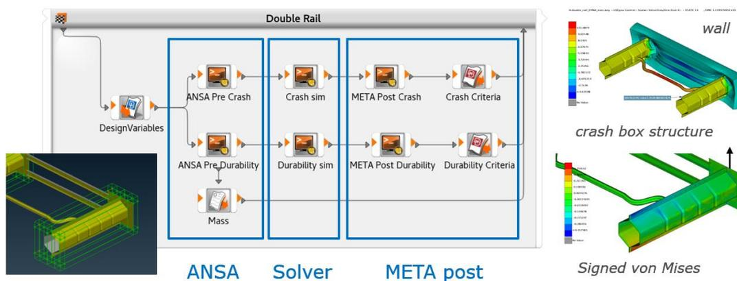
Figure 1 – MDO workflow for direct optimization, illustrating the coupling of two disciplines covering individual integrations for pre-processing, simulation and post-processing.
