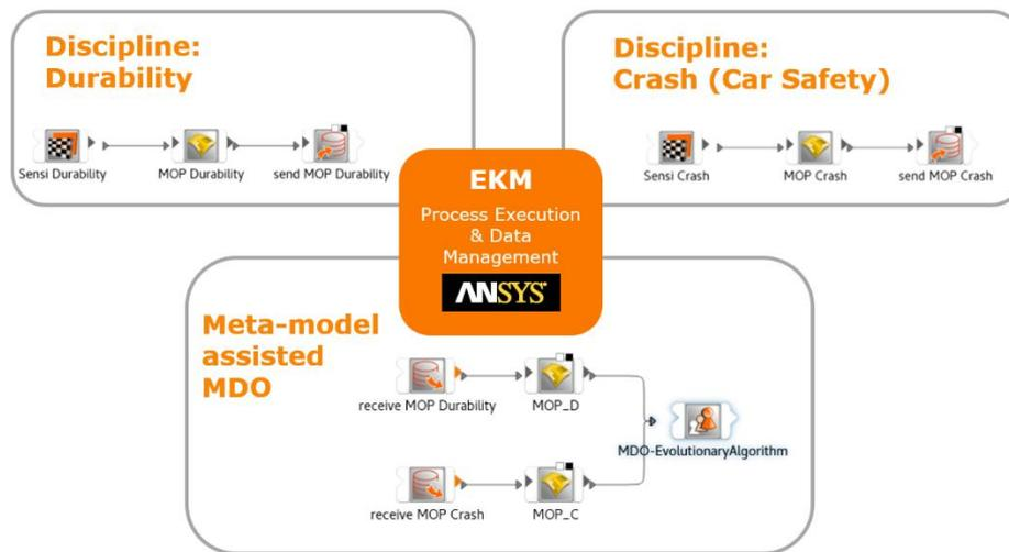
Figure 2 – Conceptual view on the exchange of meta-models via EKM (Simulation Data and Process Management) solution between individual disciplines and the meta-model assisted MDO process.
