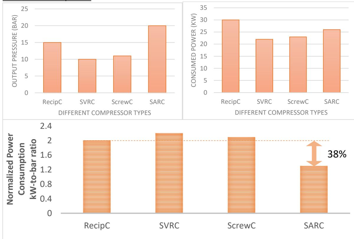
Figure 9 – Comparison of different types for medium size applications
