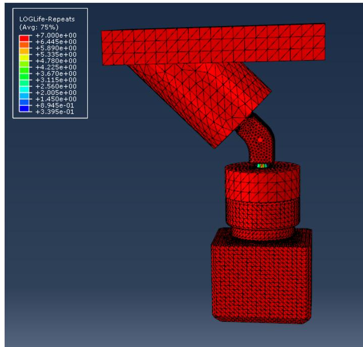
Figure 6: Log Life contour of the Implant
