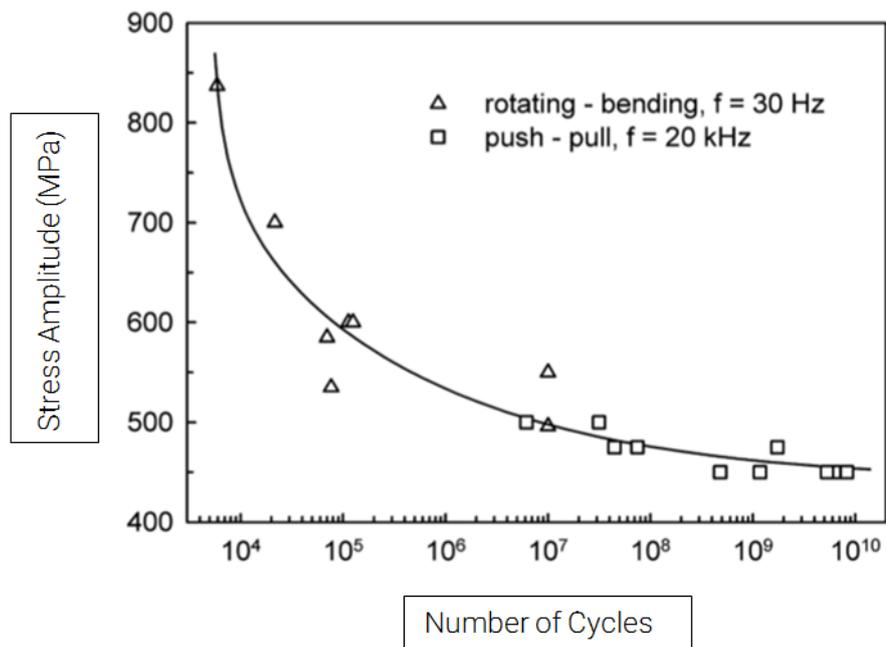
*Figure 5: S-N curve of Ti-6Al-4V*
