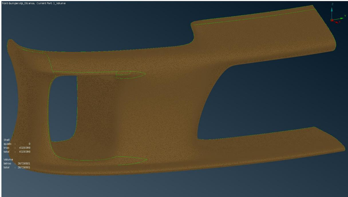
Figure 3: Meshed bumper CAD model (front view)
