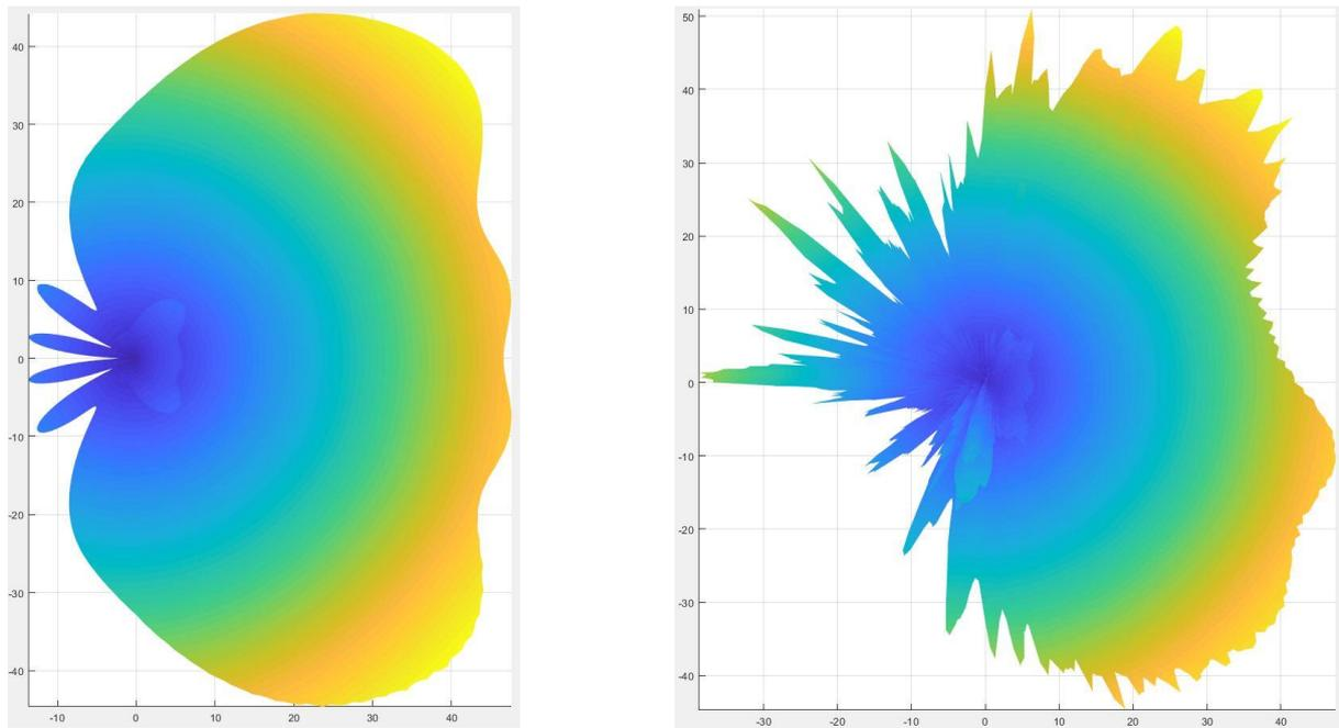
**Figure 5: Top view (in azimuth plane) of the 3D radiation pattern of the antenna in free space (left) and behind the bumper (right)**
