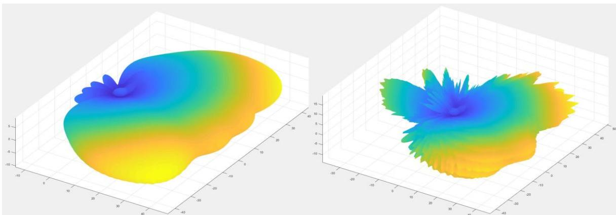
Figure 4: 3D radiation pattern of the antenna in free space (left) and behind the bumper (right)
