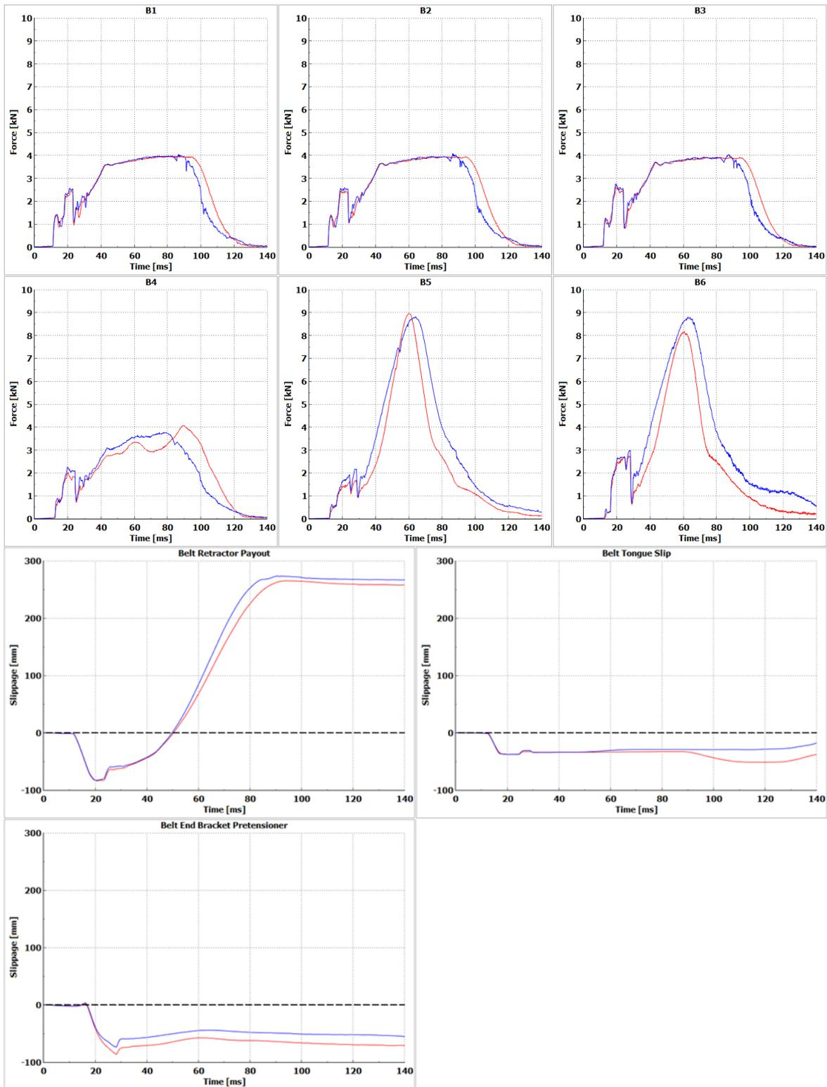
Figure 13 – Comparison of belt outputs between THUMS (represented in blue) and THOR-Reclined (represented in red) simulation models.
