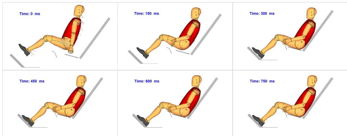
Figure 7 - ATD positioning (pre)simulation. The environment elements (in grey) start 150 mm away from their original position and are repositioned during the first stage of the simulation. The last 300 ms are used to reach equilibrium in the model.
