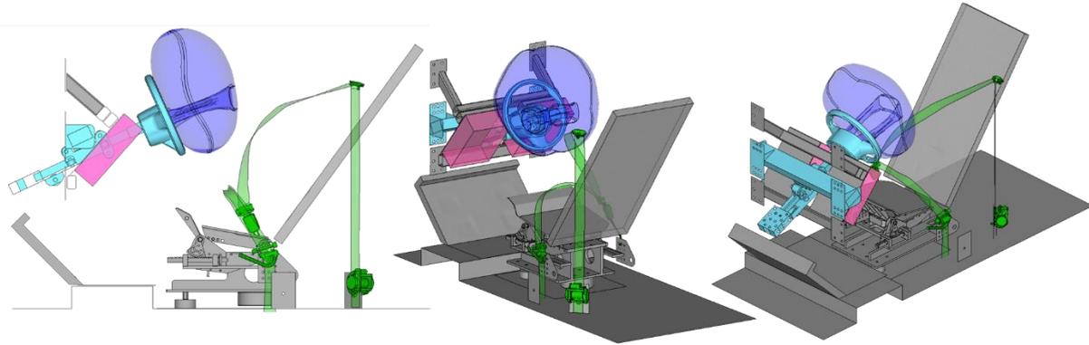
Figure 4 – The adapted generic frontal model used in the study. In grey: the semi-rigid seat, seatback, foot support, and structures. In light blue: collapsible steering column and steering wheel. In dark blue: driver airbag. In pink: knee bolster. In green: seatbelt system.
