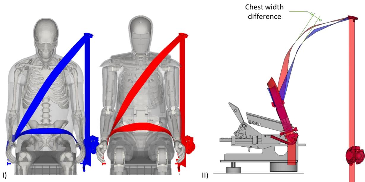
Figure 9 - Belt fit comparison of both models. The THUMS belt is presented in blue and the THOR-Reclined belt is presented in red. I) Side-by-side comparison of belt fit over each surrogate. II) Lateral view of the belt and the semi-rigid seat. A gap between both belt models can be observed due to the difference in the chest width of both models.
