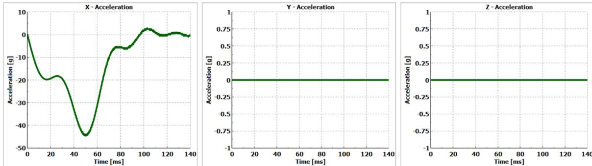
Figure 10 - Full frontal 56 km/h C2C crash pulse from EU project OSCCAR [12].
