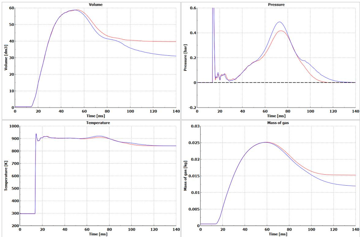
Figure 14 - Comparison of DAB outputs between THUMS (represented in blue) and THOR-Reclined (represented in red) simulation models.
