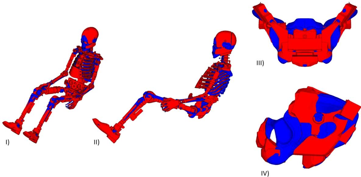
Figure 8 - Comparison of the achieved postures of the HBM (blue) and the ATD (red). I) Isometric perspective. II) Lateral view. III) Frontal view of the pelvis of both models. IV) Lateral view of the pelvis of both models.
