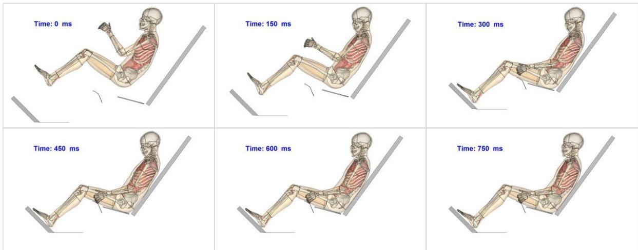
Figure 6 - HBM positioning (pre)simulation. The environment elements (in grey) start 150 mm away from their original position and are repositioned during the first stage of the simulation. The last 300 ms are used to reach equilibrium in the model.
