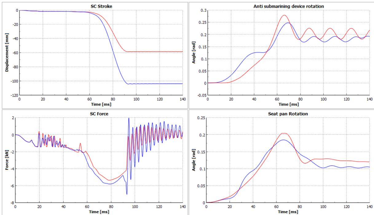
Figure 15 – Comparison of SC (Left) and Seat (Right) outputs between THUMS (represented in blue) and THOR-Reclined (represented in red) simulation models.
