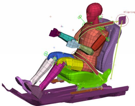
Image 1: A Seat-dummy FE model converted to a multibody model
