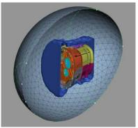
After the creation of the inner and outer boundary of the acoustic mesh, it is easy to define the volume between those two boundaries and mesh it with solid elements. Once the ACTRAN analysis has been completed, the results of the exterior noise analysis can be reviewed in the META post-processor, taking advantage of its designated post-processing capabilities.
