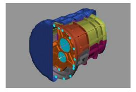
Furthermore, it represents the surface of the structure where the normal directions of the displacement results, from the modal response analysis, will act as boundary conditions in ACTRAN.
