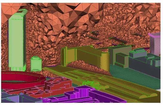
"The use of ANSA throughout the whole process of CFD model preparation allows the fast generation of high quality meshes that are necessary for reliable, accurate CFD simulations and fast results."
