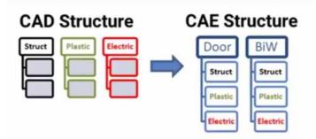
placed together. Generating this CAE structure is a demanding and error prone task for which the CAD data are properly gathered, placed, and the proper materials are defined, along with the proper connectivity information.
