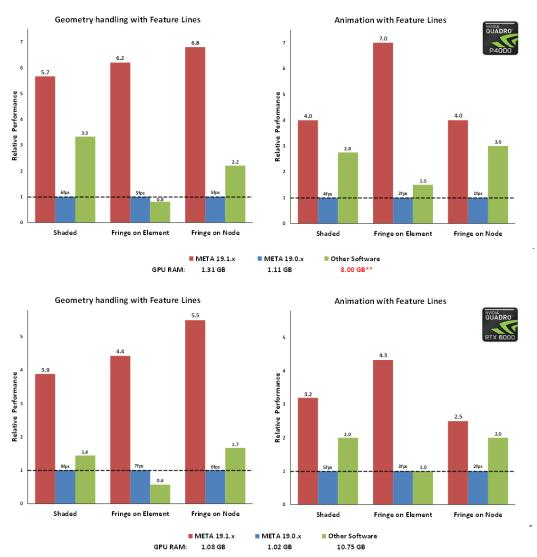
Scenario 2: 22 million elements - 16000 parts - Results: Plastic strain - Incl. Failed elements. \*\*Note: Required memory exceeds GPU memory limit leading to unpredictable performance.
