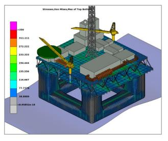
Considering the total weight of the platform at that state to be about 19200 tonnes and using a simplified model to describe only the outer surface of the hull, it is possible to find the waterline using ANSA Tank Tool by calculating the volume that the platform occupies underwater. The sea level is estimated to be 5.7 m above Hull base.
