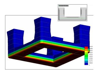
Also, gravity acceleration is applied to the whole model. By setting the inertia relief parameter in NASTRAN to -2 there is no need of SPC use in the model and the platform remains unrestrained. NASTRAN will counteract any remaining resultant force or moment by applying inertial forces induced by an acceleration field. In this way, it is possible to have a static solution.
