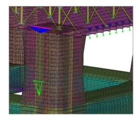
Following the same procedure as previously, the new waterline is calculated at 23.4 m above hull base. Buoyancy pressure is applied again to the new external surface below waterline. The result is a total buoyancy resultant force of 42.06\*10<sup>7</sup> N.
