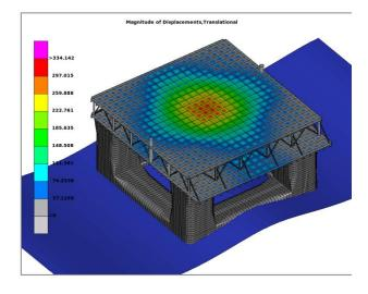
Strains, stresses and displacements are examined then in META. Critical areas with high stress values can be identified and further analysis can be done for every case. Some results are presented below.
