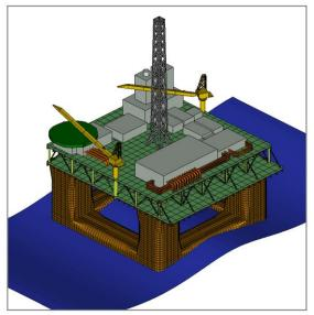
A complete model of a Semi-Submersible offshore platform, also called "SEMI", was created in ANSA with the help of the related Topology functions. The transformation tool was also used to take advantage of the symmetrical hull of the platform on X and Y axis to speed up the whole process. The whole model consists of shell elements with a variable element length according to the area of interest thus creating a rather fine meshing for a global model analysis. The model is also
