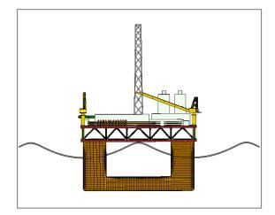
In the last case, the platform is simulated at hogging condition. The whole loading of the platform is the same as loadcase 2 but this time a trochoidal, 10 m height wave with length identical to hull's length is used. In order to position the platform on the wave ANSA special tool and "BalanceOnWave" is used then buoyancy pressure is applied again to the new external surface above water.
