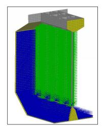
The self weight, meaning the weight of the element net, is 5487 tons. The mass of auxiliary structures that doesn't contribute to ships strength is assumed to be 4000 tons. This results to a tonnage of approximate 29800 tons. The corresponding waterline is calculated using this total weight, at a level of 11.3 meters above ships bottom, using the Tank Tool of ANSA.
